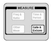
The SS7400 has two arming modes: Internal and External. Press **[Gate&ExtArm]** key until 1.000000 is displayed and the indicator light. Use **[** $\uparrow$ **]** and **[** $\downarrow$ **]** to increase and decrease values of current digit, use **[** $\leftarrow$ **]** and **[** $\rightarrow$ **]** to select digit needed to be adjust and specified range is 0.000001s to 1000s. After selecting, press **[ENTER]** to
