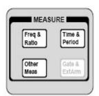
All measurement functions are realized by these three keys. Use **【Freq&Ratio】** to measure the Frequency and Frequency Ratio of CH1, CH2 and CH3. Use **【Time&Period】** key to measure Period, pulse width (Postive or Negative) and time interval. And use **【Other Meas】** key to measure count, duty cycle, phase difference and voltage.
