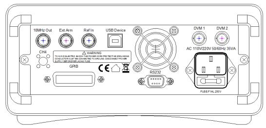
**Ref In** External frequency standard input, 5MHz or 10MHz can be selected, switch
