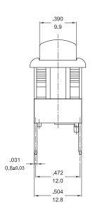
Dimensions : Inches/Millimetres Tolerances ±0.012"/0.3mm
