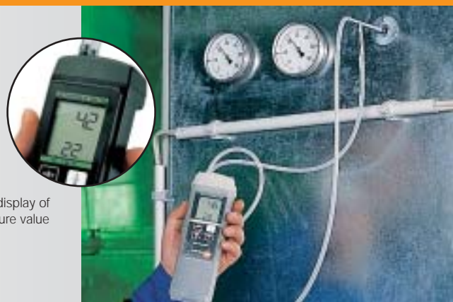
Measures flow with a Pitot tube in a ventilation duct
