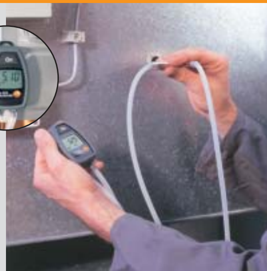
Measuring air flow with the Pitot tube
