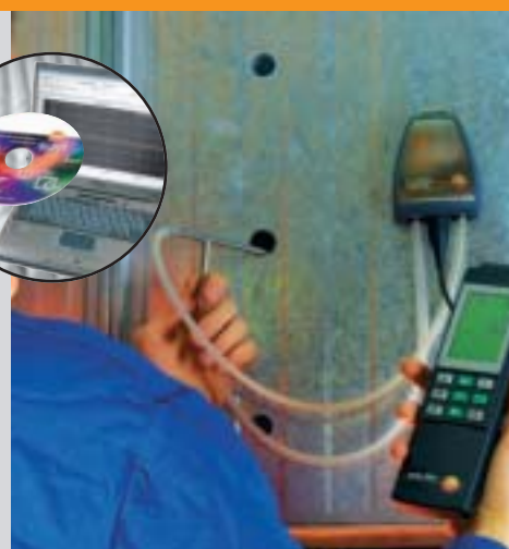
Pitot tube measurement with external 100 Pa probe
