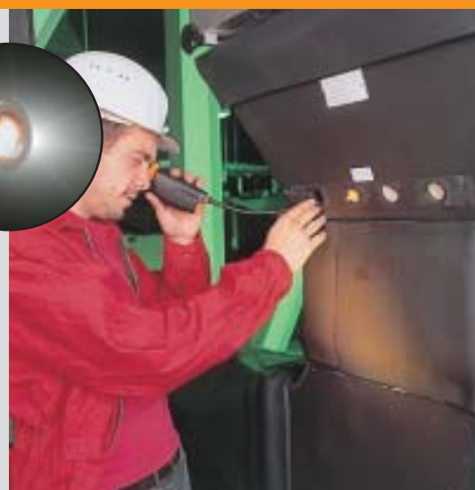
Easy detection of blocked duct channels
