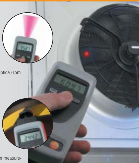
Rpm measurement on rotating parts, non-contact and mechanical
