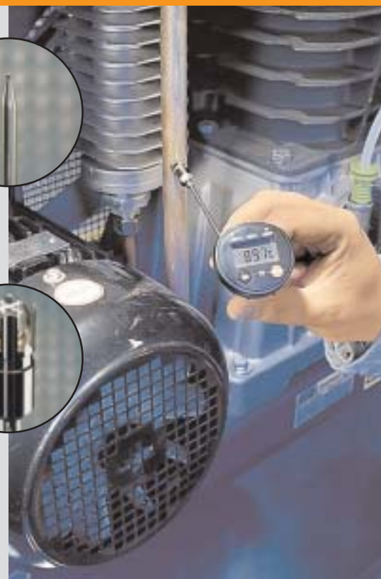
Monitoring the temperature of a refrigeration unit
