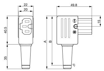
1) Cut strain relief 8 (10) mm here for 10 mm cable
