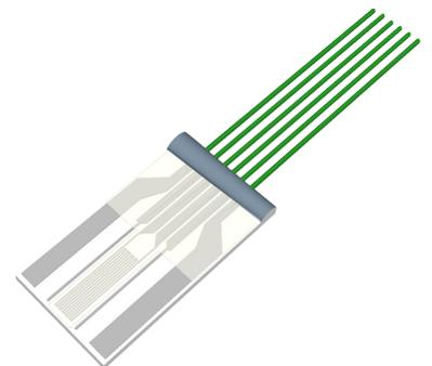
The standard IST AG LFS 117 conductivity sensor is available with either Pt/Ni wires, Ø 0.2 mm, 10 mm long or Cu/Ag wires, PTFE insulated, AWG 30.
