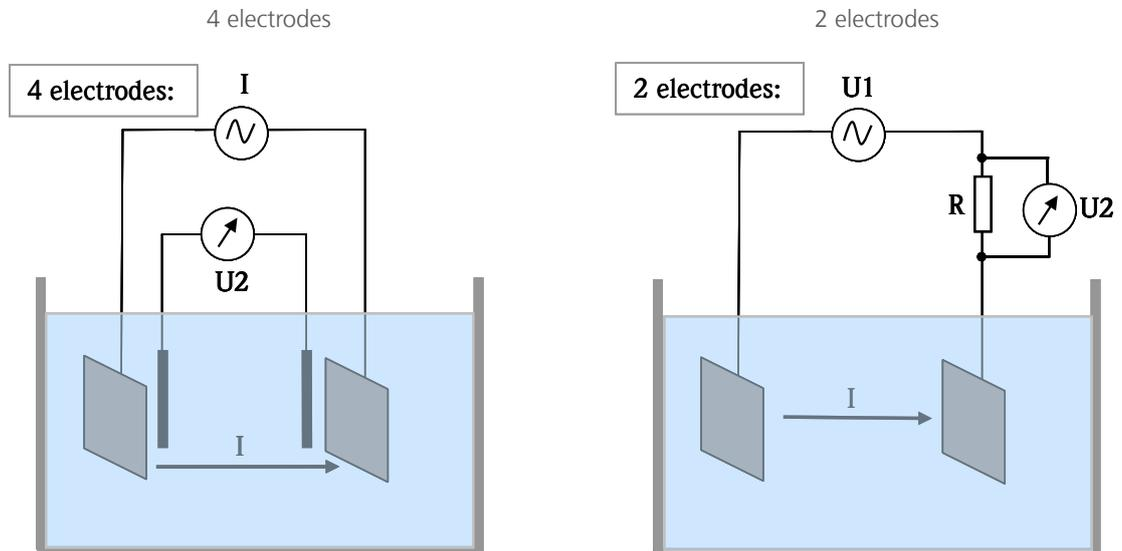
AC excitation is recommended to reduce degradation of the electrode and electrolyte.
