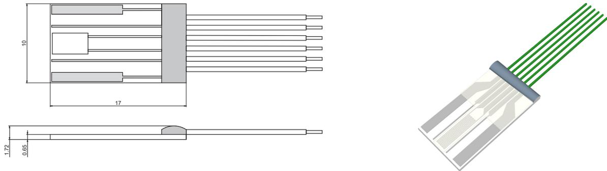
The standard IST AG LFS 117 conductivity sensor is available with either Pt/Ni wires, Ø 0.2 mm, 10 mm long or Cu/Ag wires, PTFE insulated, AWG 30.
