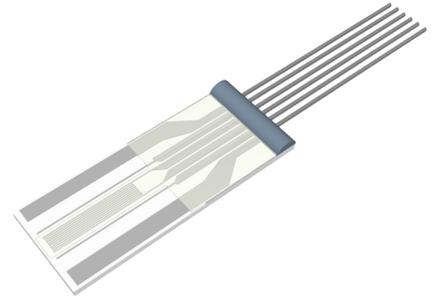
The standard IST AG LFS 155 conductivity sensor is available with either Pt/Ni wires,  $\varnothing$  0.2 mm, 10 mm long or Cu/Ag wires, PTFE insulated, AWG 30.
