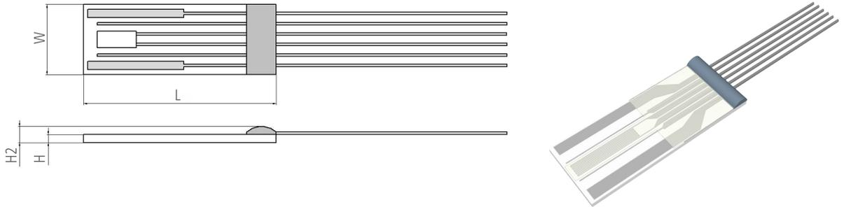
The standard IST AG LFS 155 conductivity sensor is available with either Pt/Ni wires,  $\varnothing$  0.2 mm, 10 mm long or Cu/Ag wires, PTFE insulated, AWG 30.
