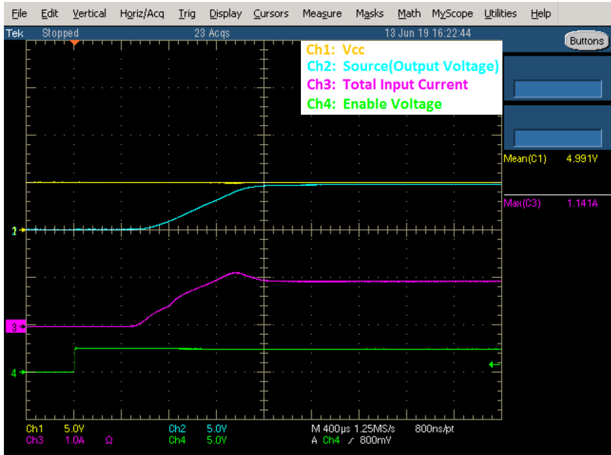
Figure 5: The eFuse turning on by ungrounding the enable pin. The controlled slew rate feature makes the output voltage to ramp up smoothly.
