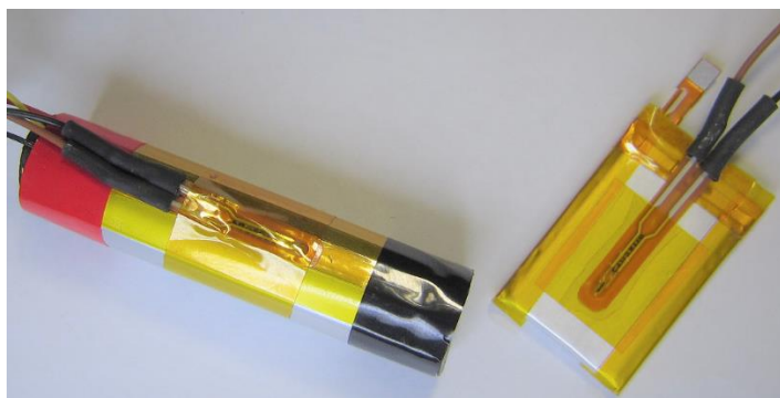
Figure 7. A LEAD TYPE THERMISTOR MOUNTING
