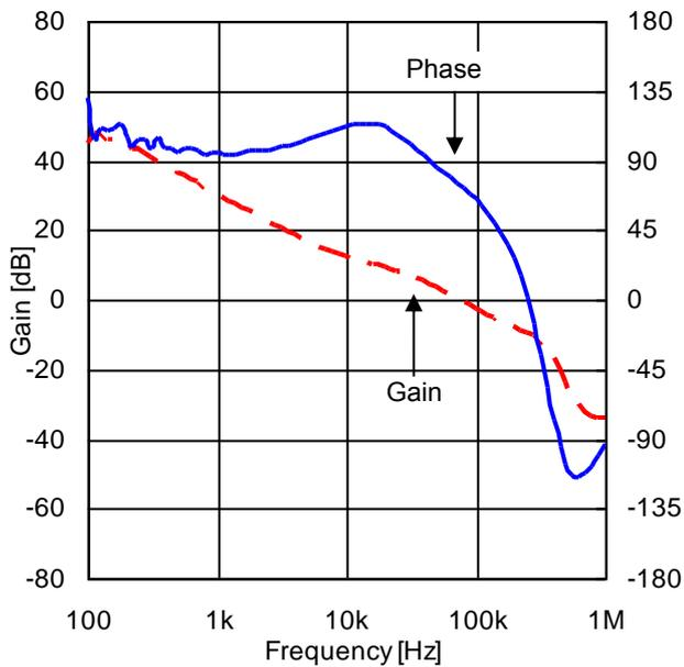
Figure 78. Frequency Characteristic (VIN = 12 V, IOUT = 0.5 A)
