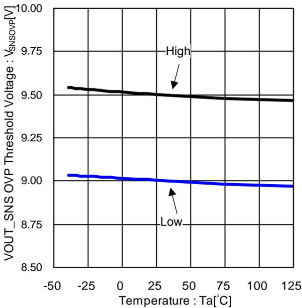
Figure 27. V<sub>OUT</sub>\_SNS OVP Threshold Voltage vs Temperature (BD9P105MUF-C)
