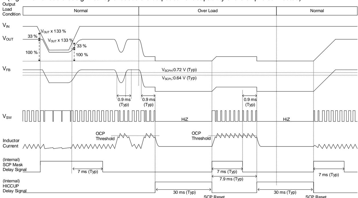
Figure 41. Short Circuit Protection (SCP) Timing Chart (BD9P105MUF-C)
