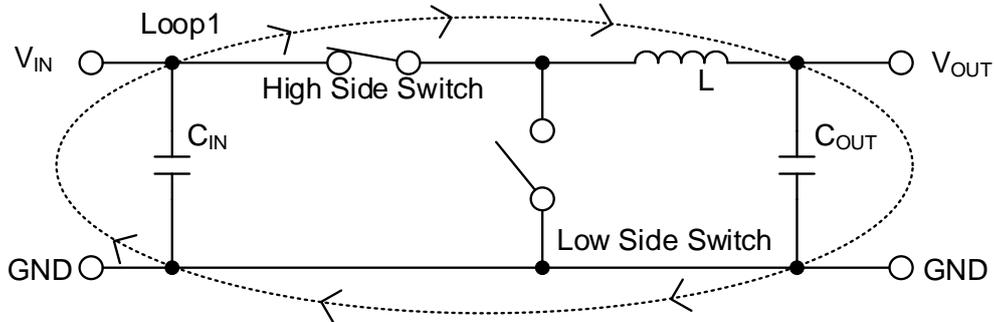
Figure 89 (a). Current Path when High Side Switch = ON, Low Side Switch = OFF
