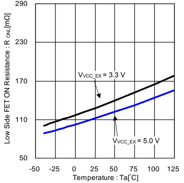
Figure 22. Low Side FET ON Resistance vs Temperature
