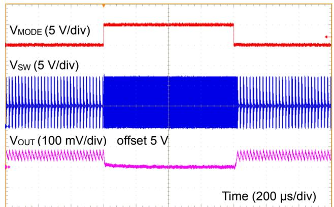
Figure 79. MODE ON/OFF Response (VIN = 12 V, IOUT = 50 mA)
