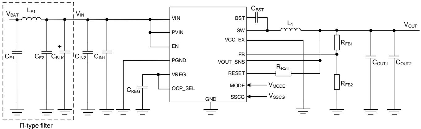
Figure 49. Reference Circuit 1
