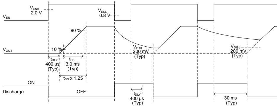
Figure 33. Enable ON/OFF Timing Chart
