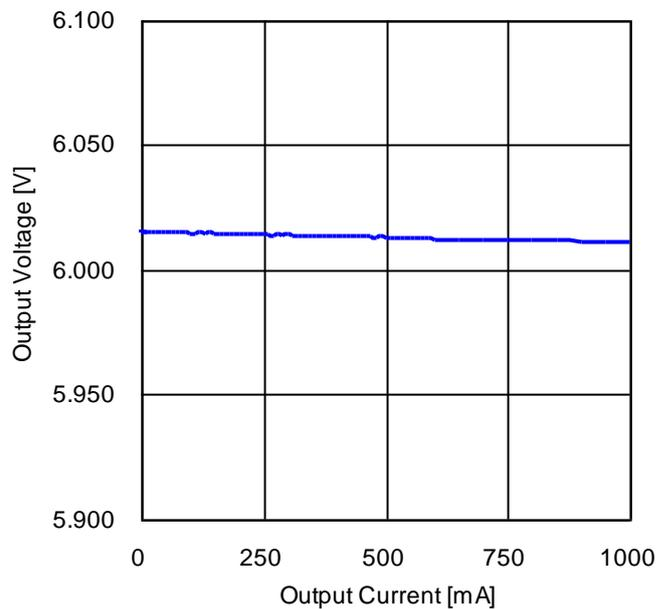
Figure 61. Load Regulation (V<sub>IN</sub> = 12 V)
