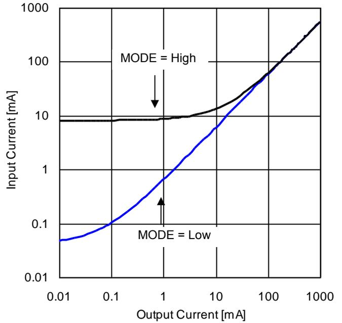
Figure 51. Input Current vs Output Current (VIN = 12 V)
