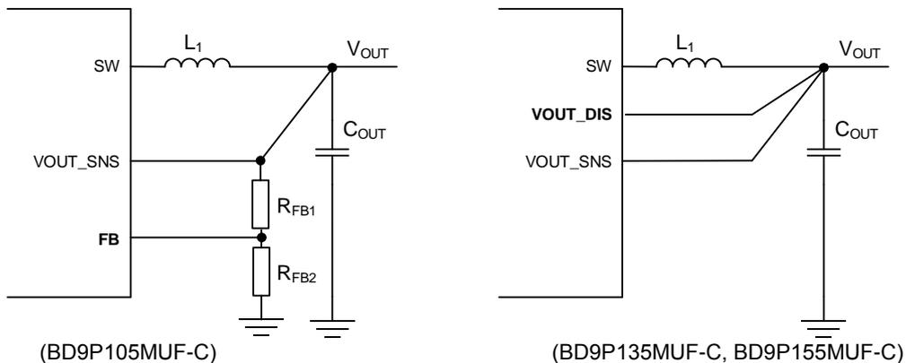
Figure 4. The difference between BD9P105MUF-C, BD9P135MUF-C and BD9P155MUF-C
