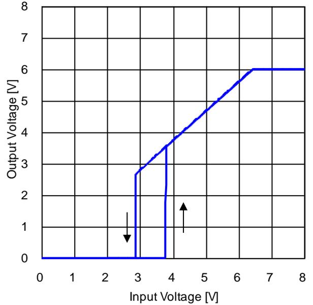
Figure 59. Output Voltage vs Input Voltage 2 (R<sub>LOAD</sub> = 6 Ω)
