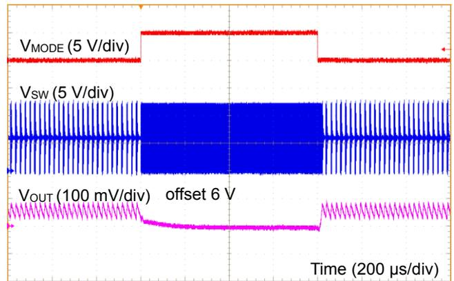
Figure 53. MODE ON/OFF Response (VIN = 12 V, IOUT = 50 mA)
