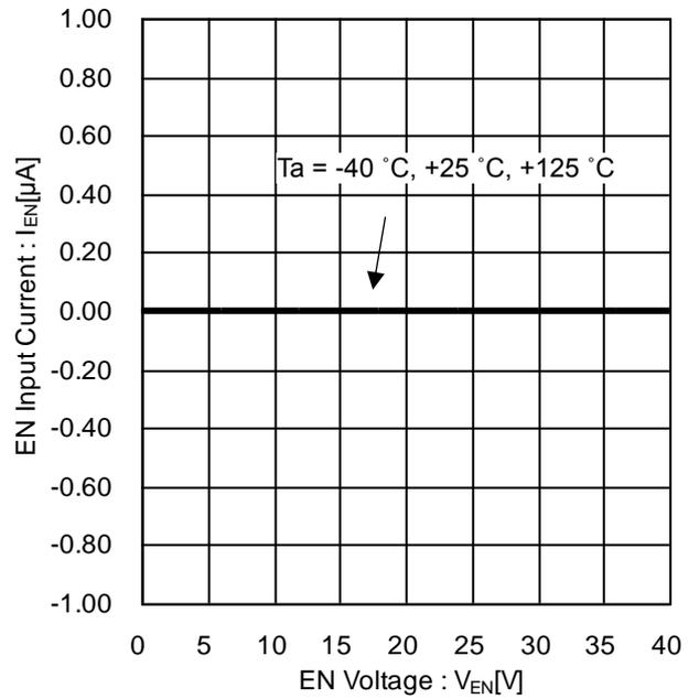
Figure 16. EN Input Current vs EN Voltage
