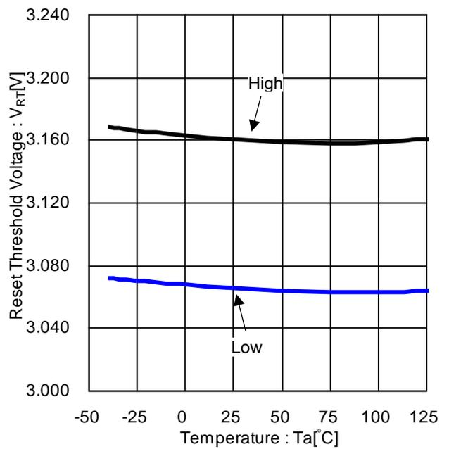
Figure 24. Reset Threshold Voltage vs Temperature (BD9P135MUF-C)
