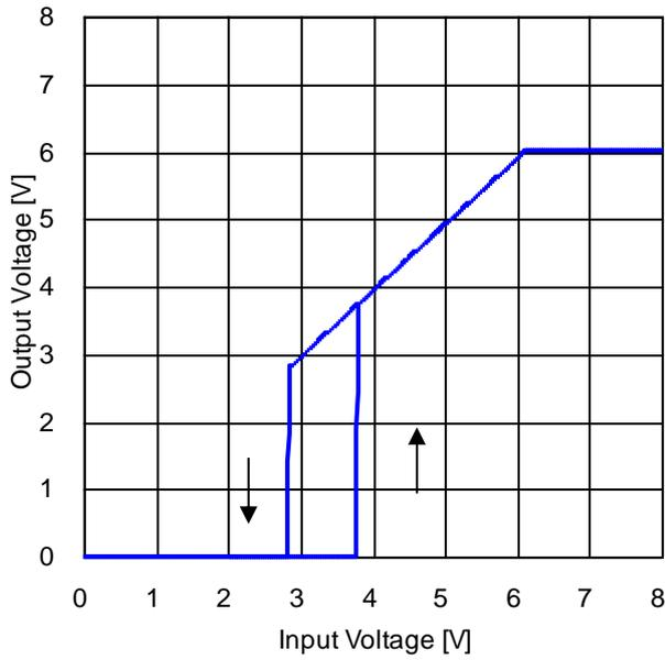
Figure 58. Output Voltage vs Input Voltage 1 (R<sub>LOAD</sub> = 600 Ω)
