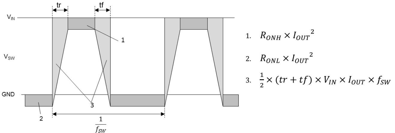
Figure 92. SW Waveform
