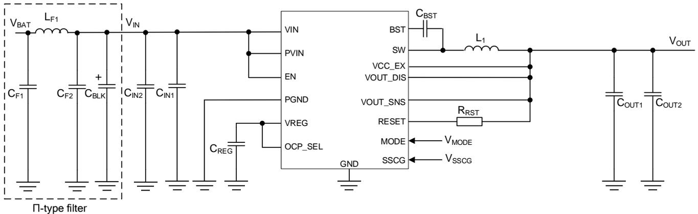
Figure 62. Reference Circuit 2
