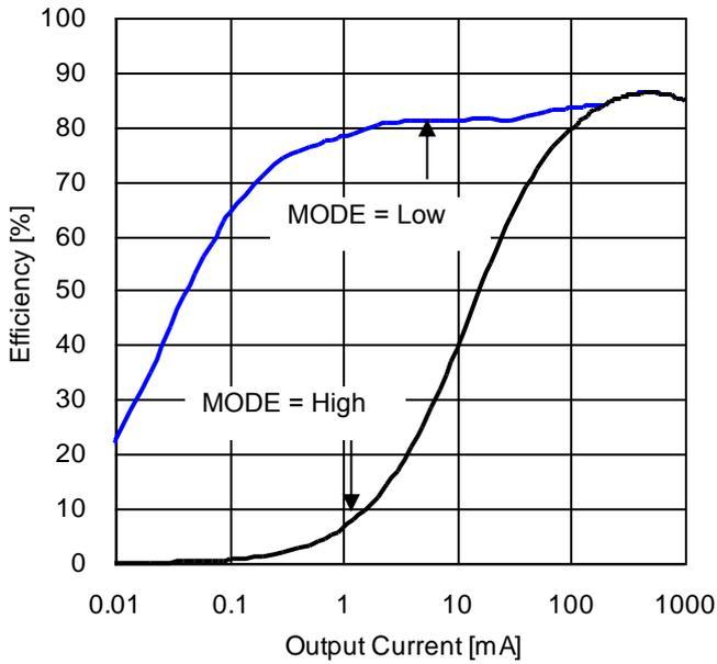
Figure 63. Efficiency vs Output Current
