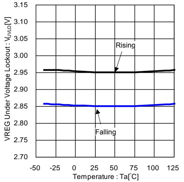
Figure 14. VREG Under Voltage Lockout vs Temperature
