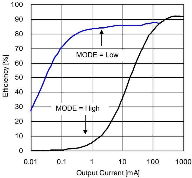
Figure 76. Efficiency vs Output Current (VIN = 12 V)
