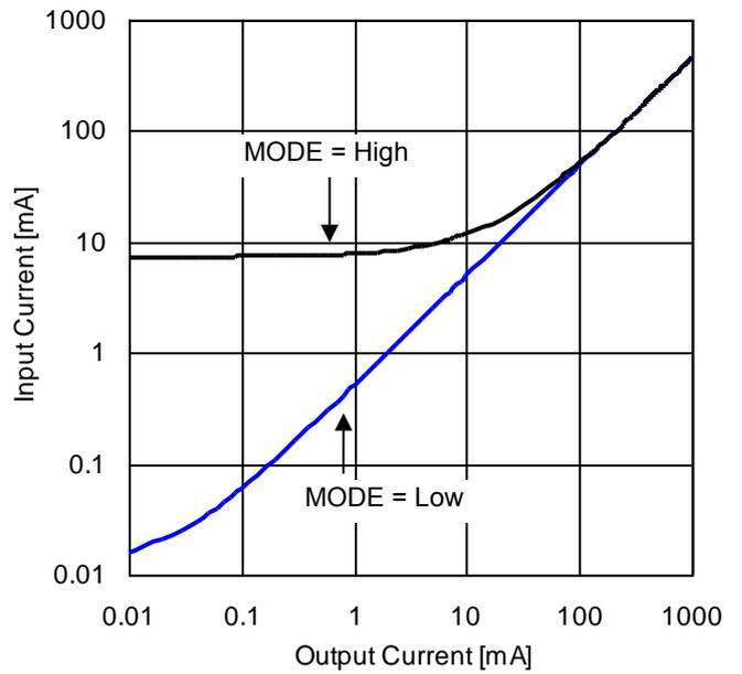
Figure 77. Input Current vs Output Current (VIN = 12 V)
