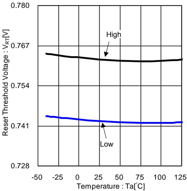
Figure 23. Reset Threshold Voltage vs Temperature (BD9P105MUF-C)
