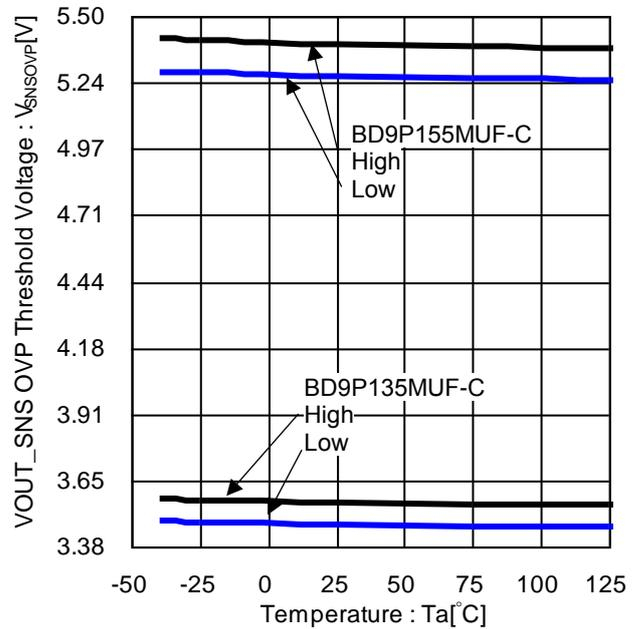
Figure 28. V<sub>OUT</sub>\_SNS OVP Threshold Voltage vs Temperature (BD9P135MUF-C/BD9P155MUF-C)
