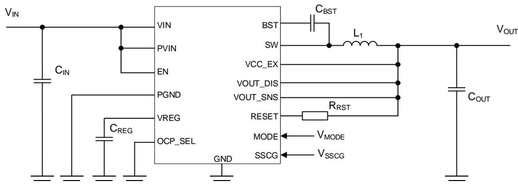
Figure 1. Application Circuit with Discharge Function (BD9P135MUF-C, BD9P155MUF-C)
