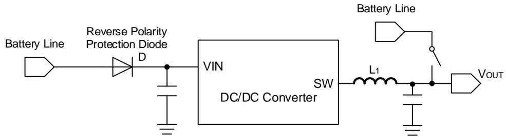
Figure 46. VOUT shorted to Battery Line
