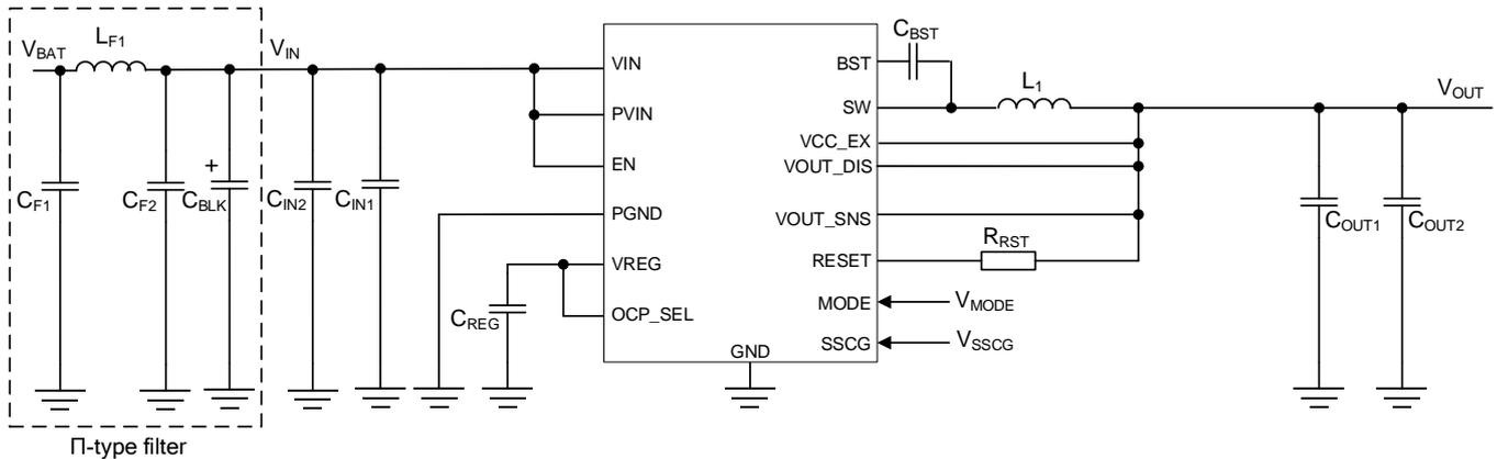
Figure 75. Reference Circuit 3
