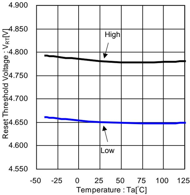
Figure 25. Reset Threshold Voltage vs Temperature (BD9P155MUF-C)
