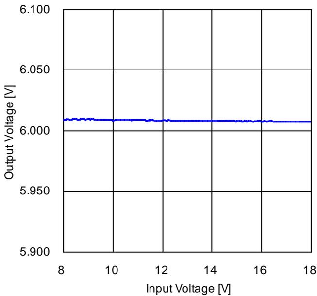
Figure 60. Line Regulation (I<sub>OUT</sub> = 1 A)
