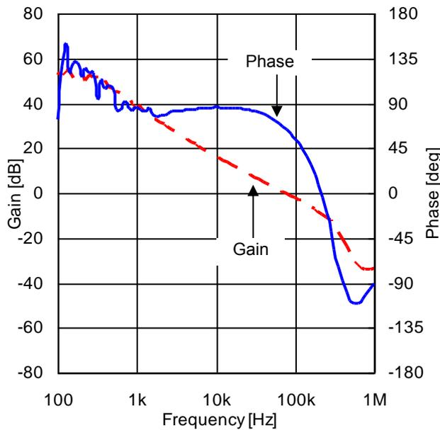
Figure 52. Frequency Characteristic (VIN = 12 V, IOUT = 0.5 A)
