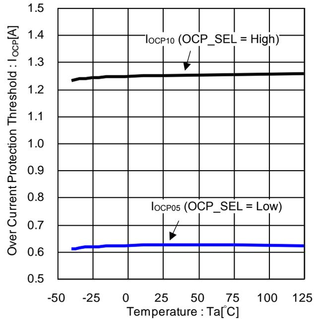
Figure 20. Over Current Protection Threshold vs Temperature
