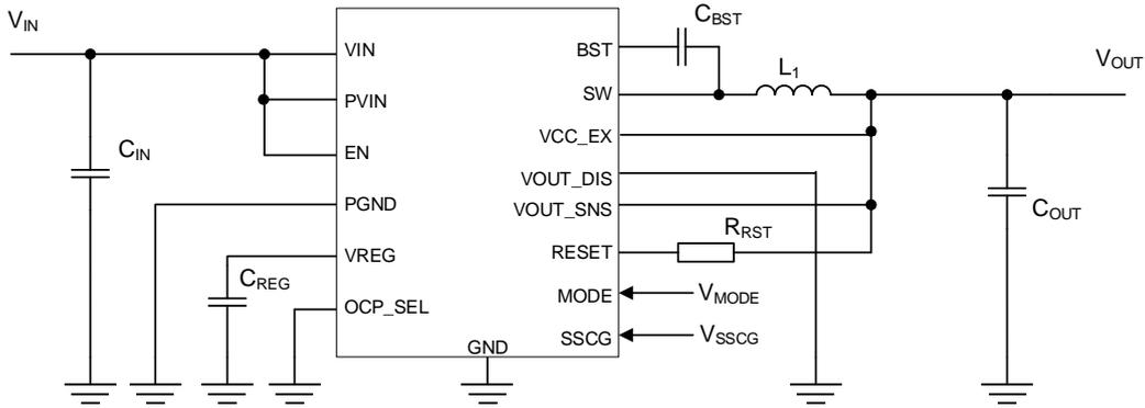
Figure 2. Application Circuit without Discharge Function (BD9P135MUF-C, BD9P155MUF-C)
