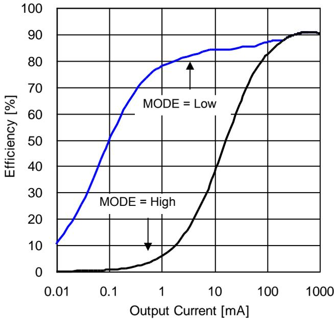
Figure 50. Efficiency vs Output Current (VIN = 12 V)
