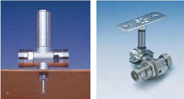
If this is not possible then the protectors should be connected to the bonding facility by a sufficiently sized grounding cable (AWG 6/16 mm<sup>2</sup> min.) as short distant as possible (0.5 m max.)
