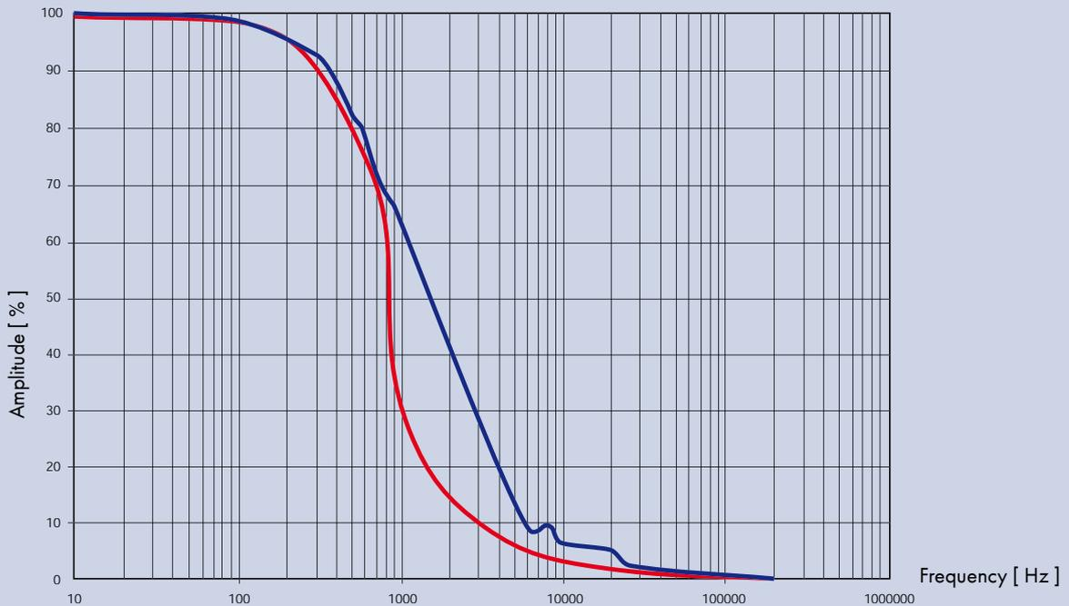
Comparison of the frequency spectra of a genuine lightning current surge (blue - according to K. Berger) and a test current surge 10/350  $\mu$ s (red - according to IEC 61312-1)
