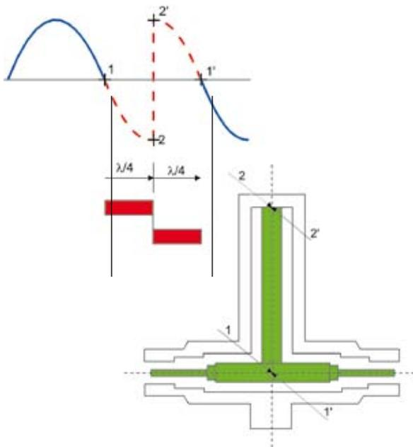
In regular operation, the RF signal reaches the entry of the shorting stub (shown here as point 1). It then runs along the shorting stub up to the short (point 2). This corresponds to a 90° phase shift. At the short, the signal is reflected (point 2') – a sudden phase shift of 180° is created – and flows back to the start of the
