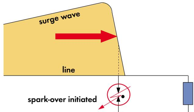
The voltage across the surge protection capsule then rises very rapidly. When the dynamic spark-over voltage has been reached, the surge protection capsule will ignite and become conductive. At this moment, the voltage across the surge protection capsule (called the glow-arc voltage) is between 72 and 90V. This collapses to 10 – 20V (called the arc voltage), as the current rises. The dynamic spark-over voltage of the surge protection capsule is a function of the pulse rise time.
