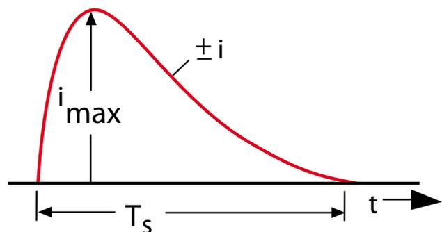
2) Positive or negative lightning current pulse as 1), with subsequent long-duration current of about 100 A during a period of less than 500 ms ( $T_1$ ).
