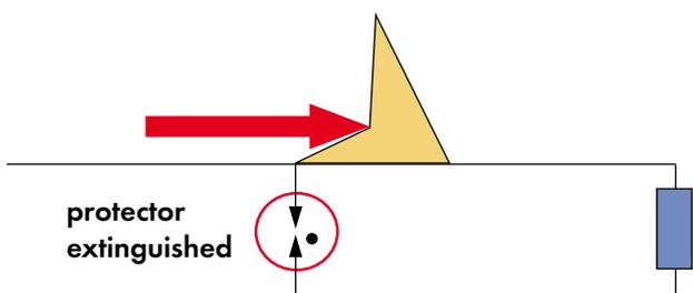
After the interference has subsided, the surge protection capsule is extinguished, reverting to its original high-ohmic condition.
