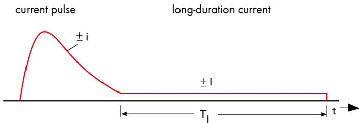
lightning current pulse according to 1) followed by subsequent lightning currents up to 10 kA. The break times between the lightning current pulses are shorter than 100 ms ( $T_p$ ).
