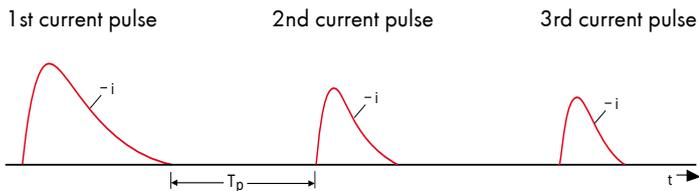
4) Sequence of negative lightning currents according to 3), with integral long-duration current according to 2).
