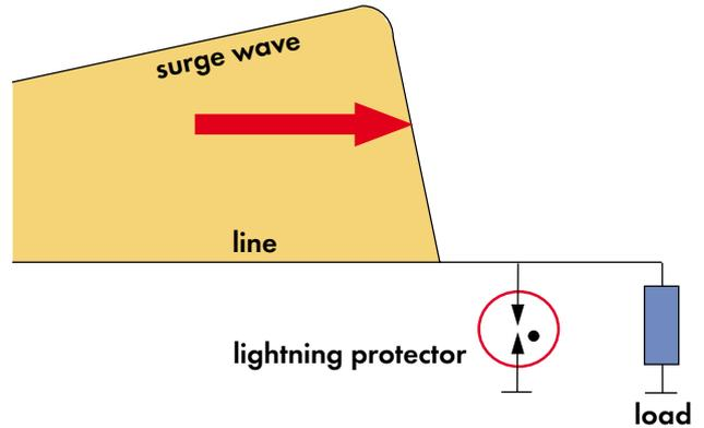
«Load» stands for the electronic equipment that has to be protected. The surge protection device is symbolized by the discharge capsule.
