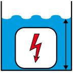
temporary immersion (test 1 m, 30 min.)
