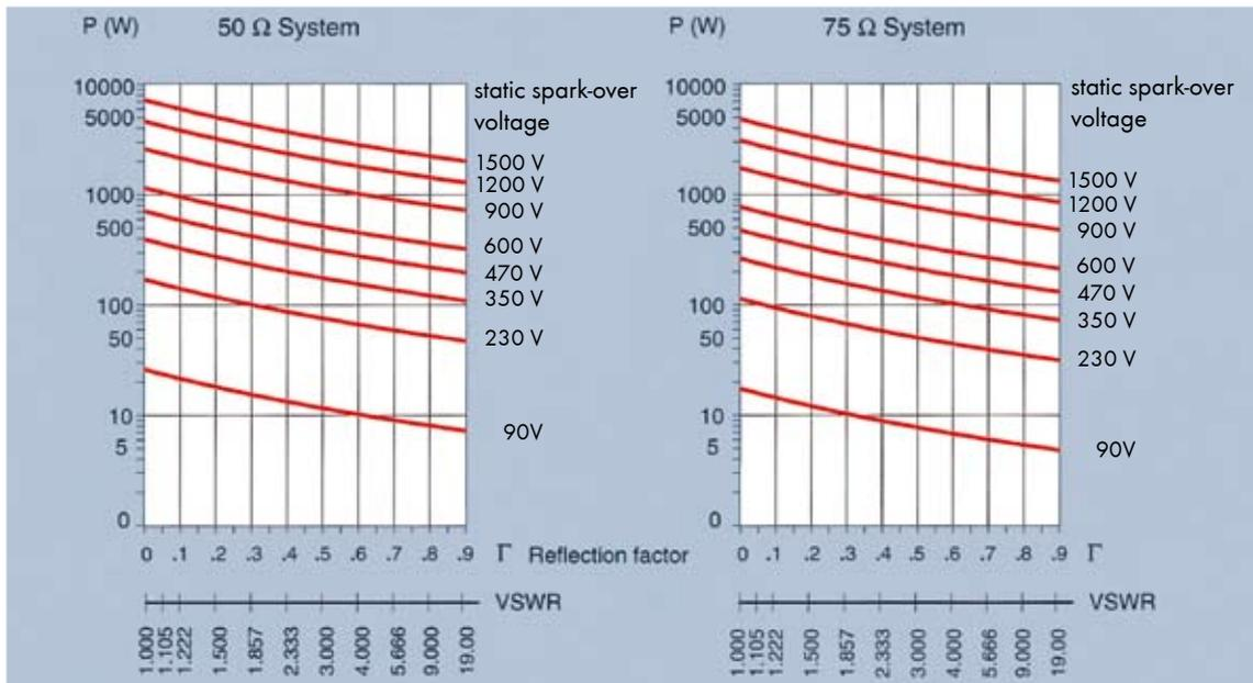
Diagrams of permissible RF power (CW or PEP) for 50  $\Omega$  and 75  $\Omega$  systems
