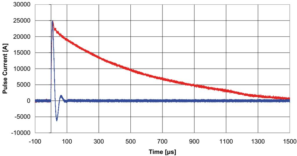
Comparison of the test pulses 10/350  $\mu$ s (real lightning current – red) and 8/20  $\mu$ s (blue) concerning electrical charge and specific energy (destructive potential) for equal current amplitudes
