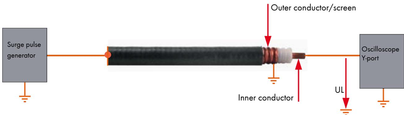
Such a surge suppressor is not only required due to the leftover residual pulse of the gas capsule lightning protector, but also due to magnetic coupling into the possible loop which the antenna cable length between the lightning protector and the equipment is part of (within zone LPZ 1). This is illustrated by the following:
