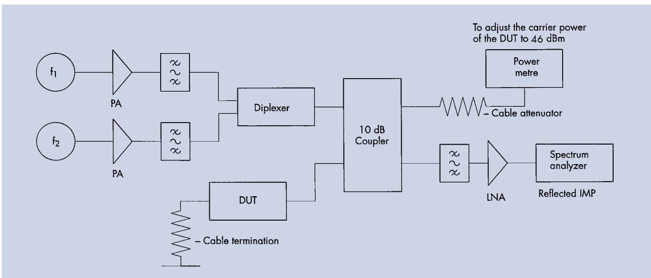
Tests can be performed for the following bands: TETRA, AMPS/North American Digital Cellular, GSM900/1800, PCS1900 and UMTS
