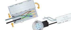
8. If required, the WAGOBOX 221-4 can be fitted to a surface using the WAGOBOX mounting button feature. (sold separately, part No. 51009130 pack of 10)
