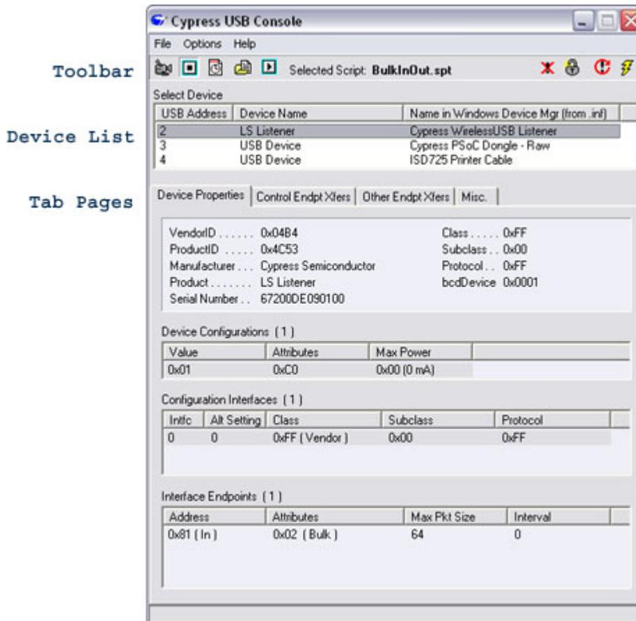
The **Configuration Interfaces** section lists all the interfaces (including alternate interfaces) exposed by the device. Clicking on an interface in the list automatically selects that interface and causes its endpoints to be displayed in the **Interface Endpoints** list.
