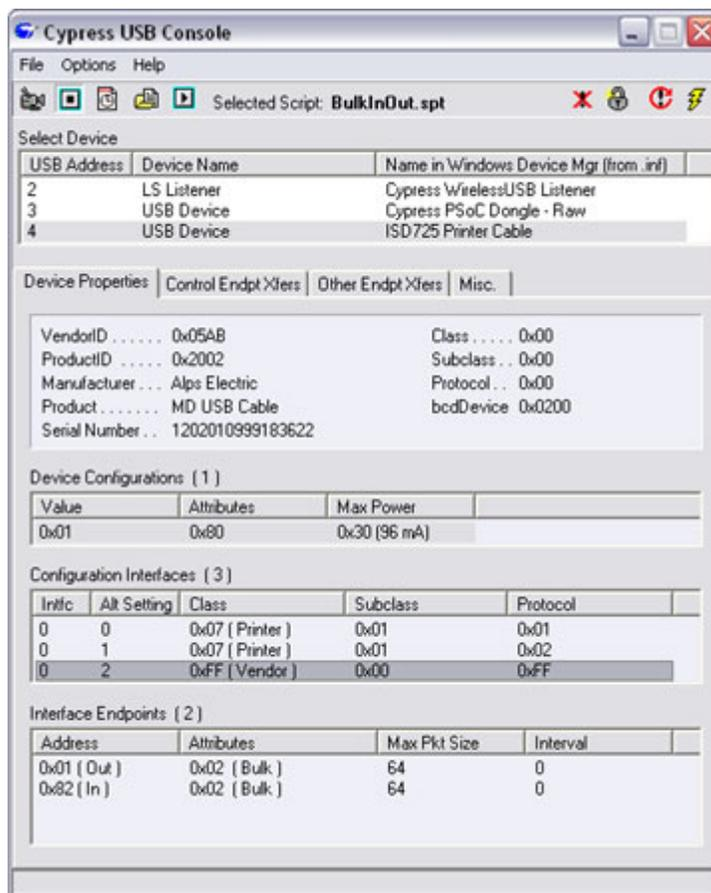
NOTE: A properly functioning Windows USB driver stack will report each primary interface as a separate USB device. So, USB devices that report multiple primary interfaces will actually show-up as multiple USB devices in the USB device list (one for each interface).
