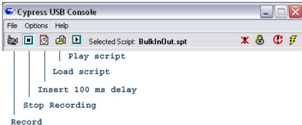
A recording session is started by clicking on the camera icon in the toolbar. The status bar at the bottom of the Console window will display "Recording . . ." in red.
