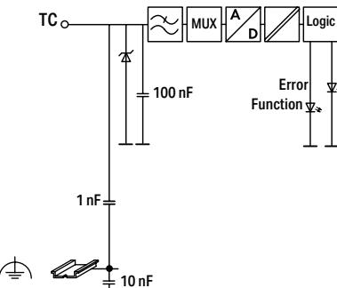
The 750-498 I/O Module measures either voltages (mV) in the field or analyzes thermocouples.
