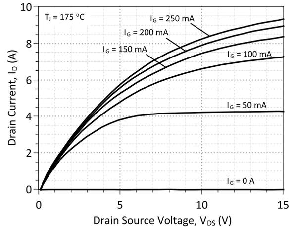
**Figure 2: Typical Output Characteristics at 175 °C**
