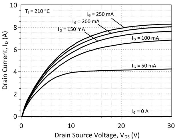
**Figure 3: Typical Output Characteristics at 210 °C**
