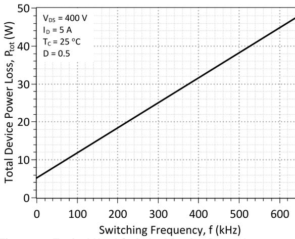
**Figure 13: Typical Hard Switched Device Power Loss vs. Switching Frequency<sup>2</sup>**
