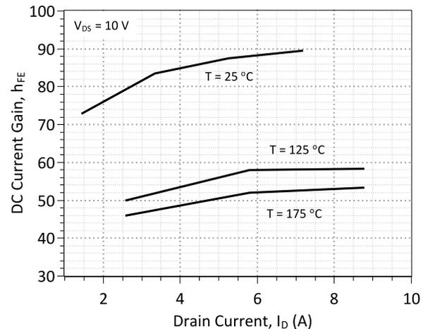
**Figure 6: DC Current Gain vs. Drain Current**
