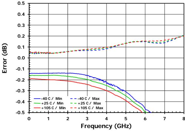
Figure 17. Step Accuracy vs Attenuator Setting [LSB = 0.25dB]
