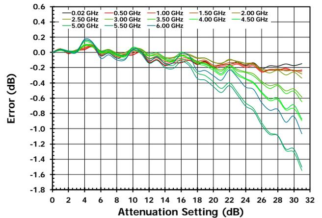
Figure 16. Worst Case Step Accuracy vs Frequency [LSB = 0.25dB]
