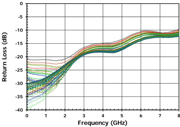
Figure 8. Output Return Loss vs Frequency [All States]
