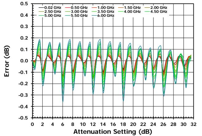
Figure 20. Worst Case Step Accuracy vs Frequency [LSB = 1.00dB]
