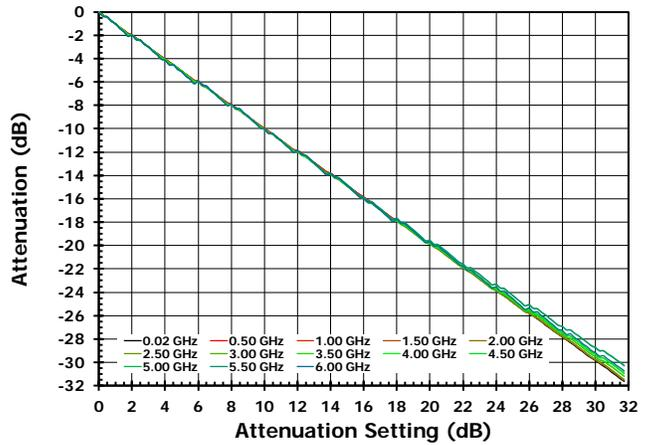
Figure 26. Insertion Loss vs Frequency [0dB]
