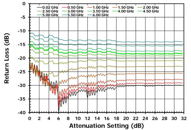
Figure 9. Output Return Loss vs Attenuator Setting
