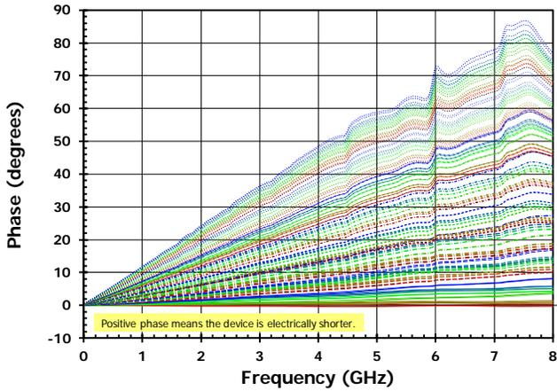
Figure 23. Relative Insertion Phase vs Attenuator Setting
