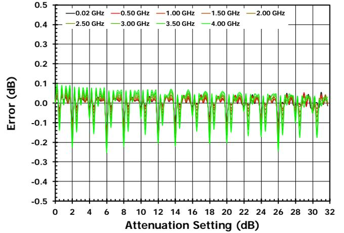
Figure 18. Worst Case Step Accuracy vs Frequency [LSB = 0.50dB]
