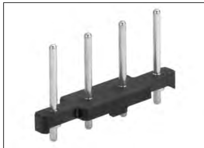
4-contact male header for THR-soldering; grid 5.75 mm
