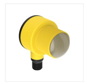
T30R R-GAGE Series Radar Sensor Range 15 m; Input 10-30 V dc 0-10 V Analog, 1 NPN/PNP Configurable with IO Link 5 Pin Euro (M12) Quick Disconnect
