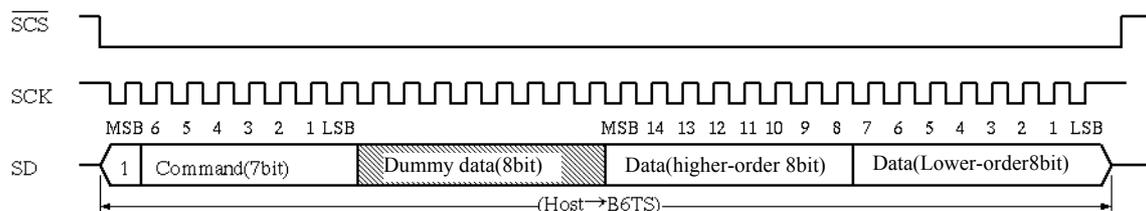
If data communication is performed during normal measurement mode, the measurement operation stops while the data is communicated.
