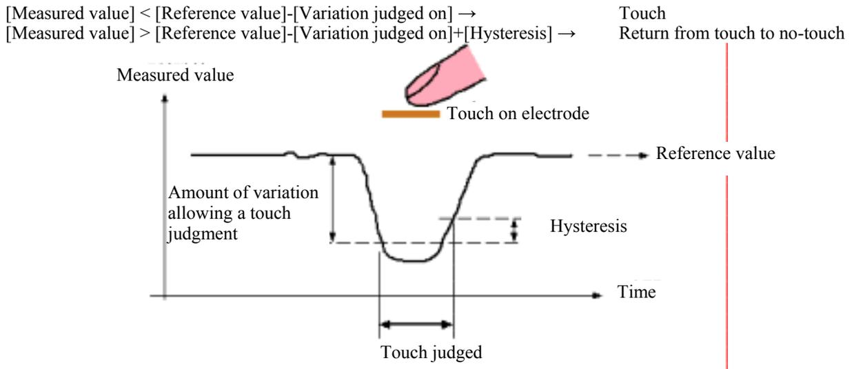
Even in the touched state, the measured value changes according to variation in the environment (output drift). The chip is provided with an automatic drift-correction function, which can cancel mild changes of the measured value due to variation in the environment (drift correction function). It is possible to select whether or not to execute drift correction in setup mode.
