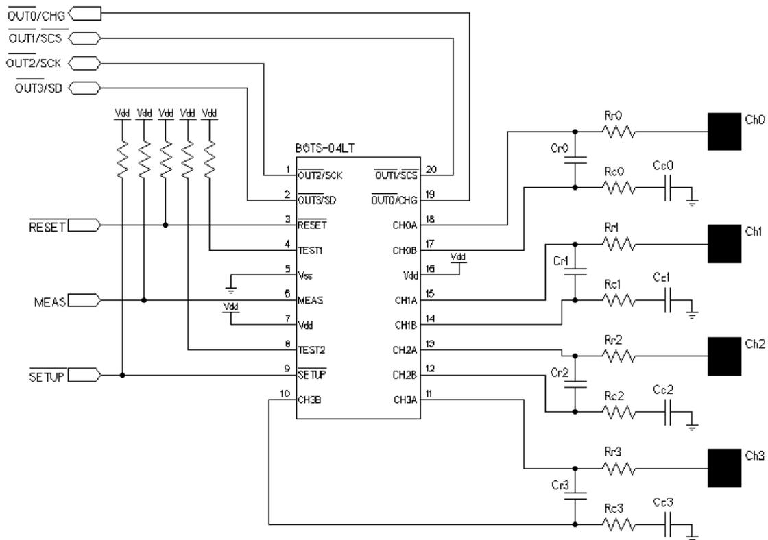
Note 1: Connect  $R_r$ ,  $C_r$ ,  $R_c$ , and  $C_c$  to each touch electrode, as shown in the above figure. Refer to the design tool (B6TWWorkbench) for their actual values.
