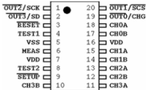
Note 1: Pins TEST1, and TEST2 are used for testing during manufacture of the IC. When using these pins, connect them to VDD through a pull-up resistor.
