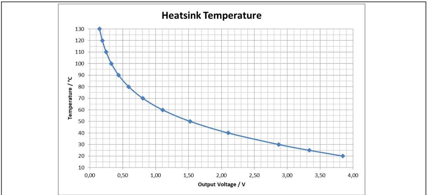
Figure 22 Heatsink temperature output
