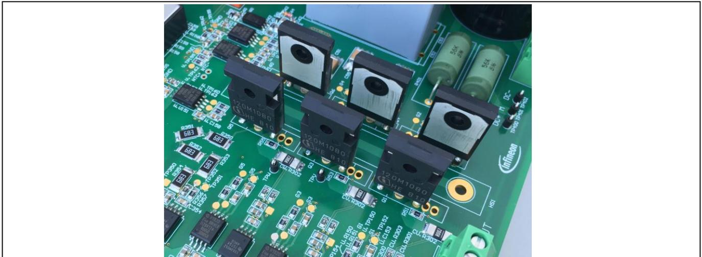
**Figure 3** View of the power stage without heatsink
