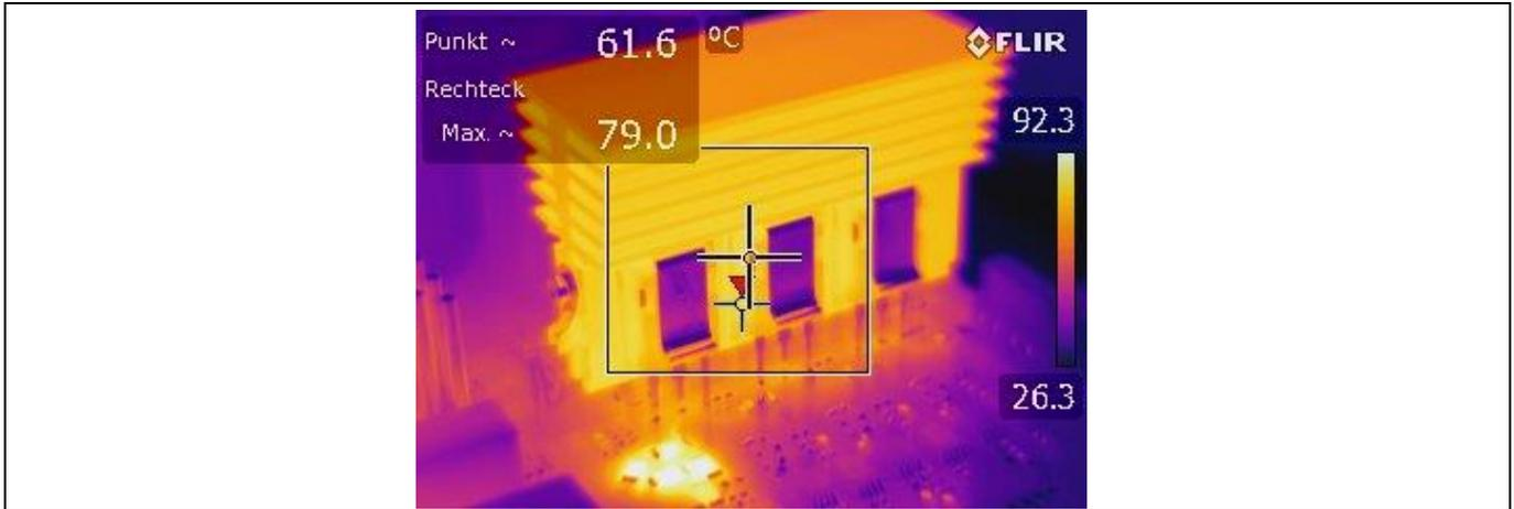
Figure 30 Thermal image the left power MOSFETs
