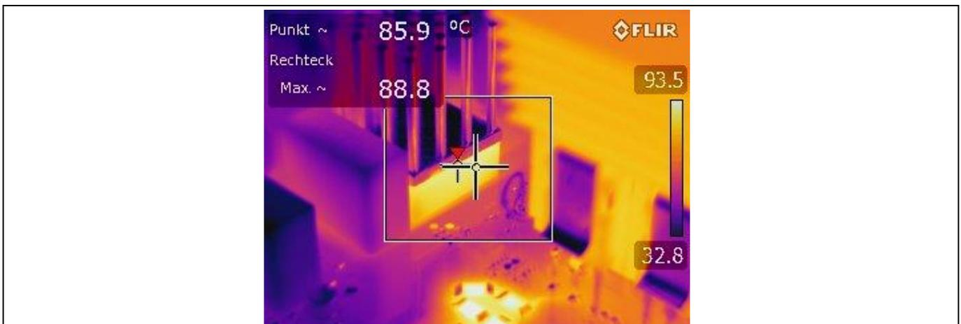
Figure 32 Thermal image of the input rectifier
