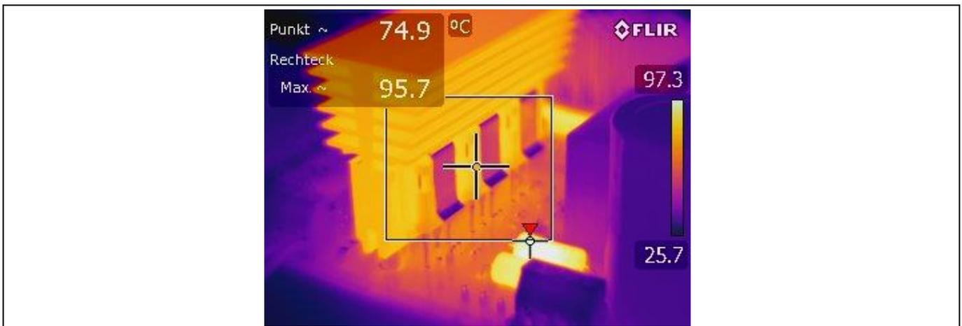
Figure 31 Thermal image of right power MOSFETs (hotspot at the capacitor's balancing resistors)
