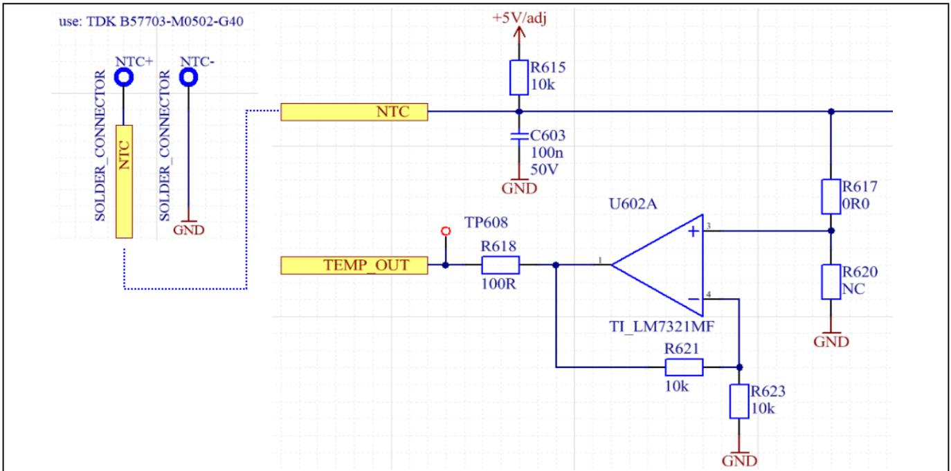
Figure 21 Evaluation circuit for NTC measurement
