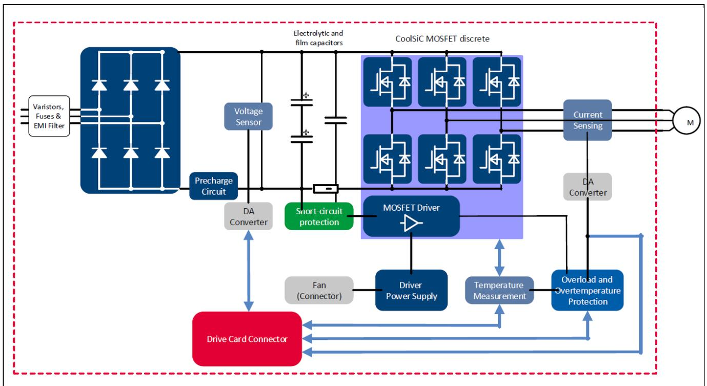
Figure 1 The block diagram of the EVAL-M5-IMZ120R-SIC
