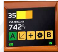
Tip temperature displayed on large color screen.
