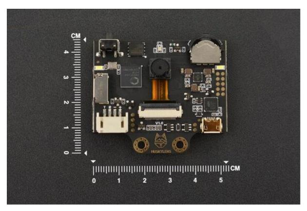
Gravity: HuskyLens is an easy-to-use Al machine vision sensor. It's equipped with multiple functions such as face recognition, object tracking, object recognition, line tracking, color recognition and tag(QR code) recognition.
