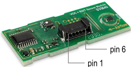
**Table 4** Pin assignment of the Molex connector. Pin colors match with assignment of the jumper wire cables, which is delivered together with the SEK-SVM40.
