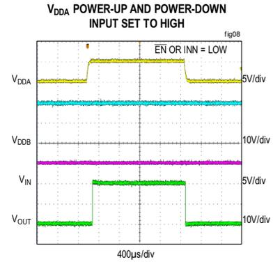
Figure 8.  $V_{DDA}$  Undervoltage Lockout Behavior (Input High)
