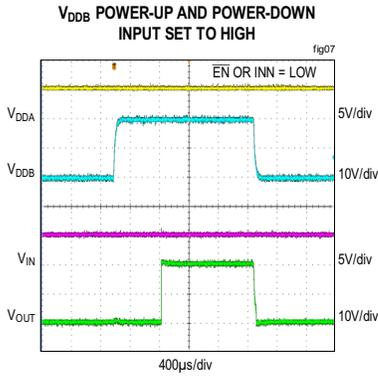
Figure 7.  $V_{DDB}$  Undervoltage Lockout Behavior (Input High)
