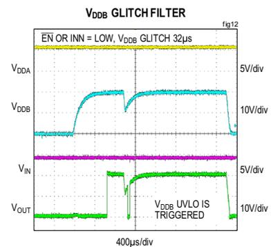
Figure 12.  $V_{DDB}$  Undervoltage Lockout Glitch Filter, UVLO Triggered
