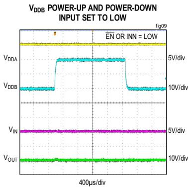
Figure 9.  $V_{DDB}$  Undervoltage Lockout Behavior (Input Low)
