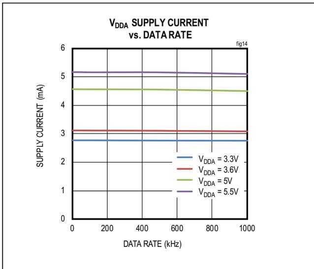
Figure 14.  $V_{DDA}$  Supply Current vs. Data Rate (typ)
