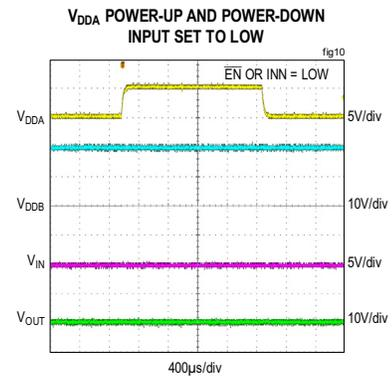
Figure 10.  $V_{DDA}$  Undervoltage Lockout Behavior (Input Low)
