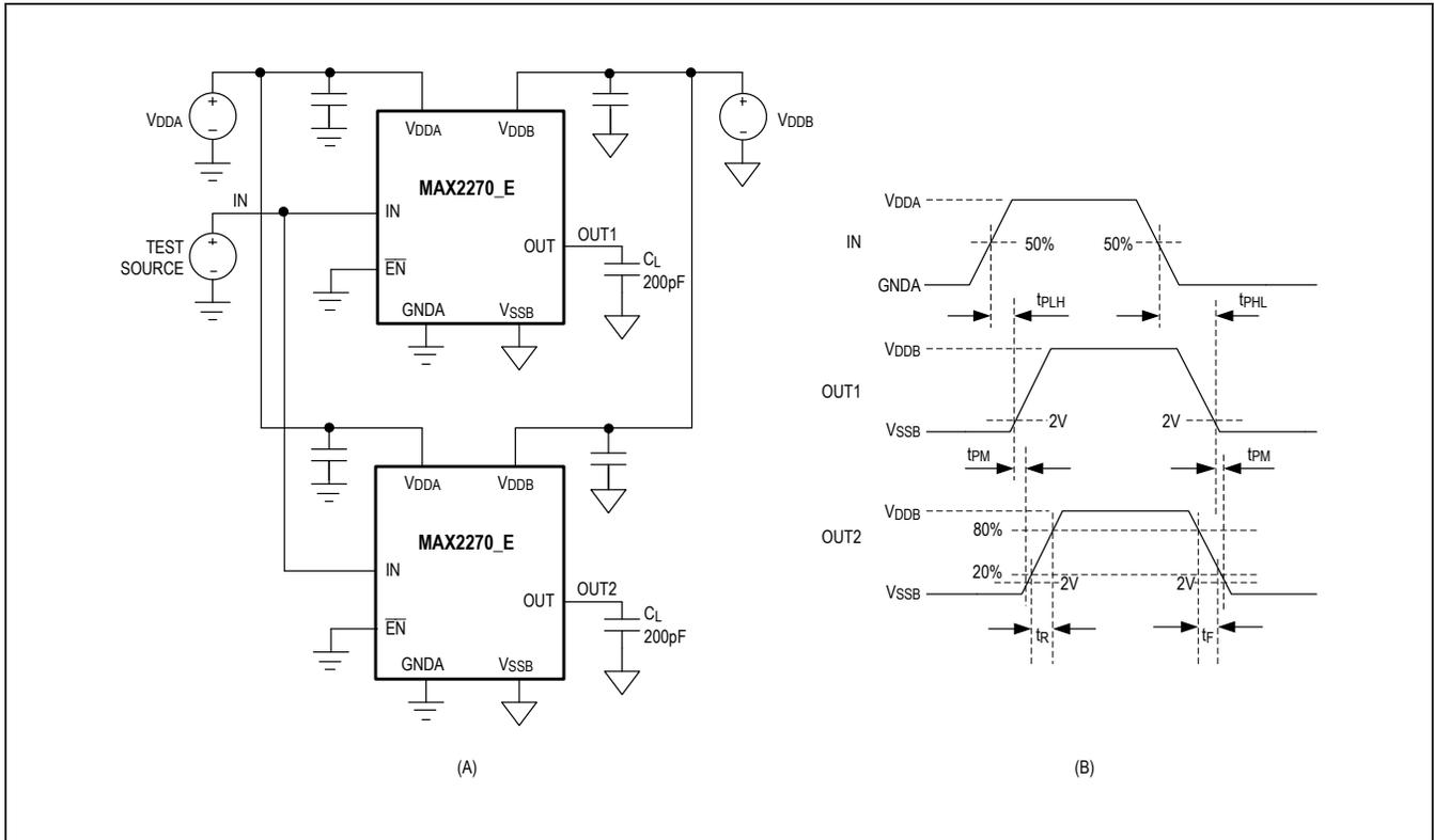
Figure 3. Test Circuit (A) and Timing Diagram (B)
