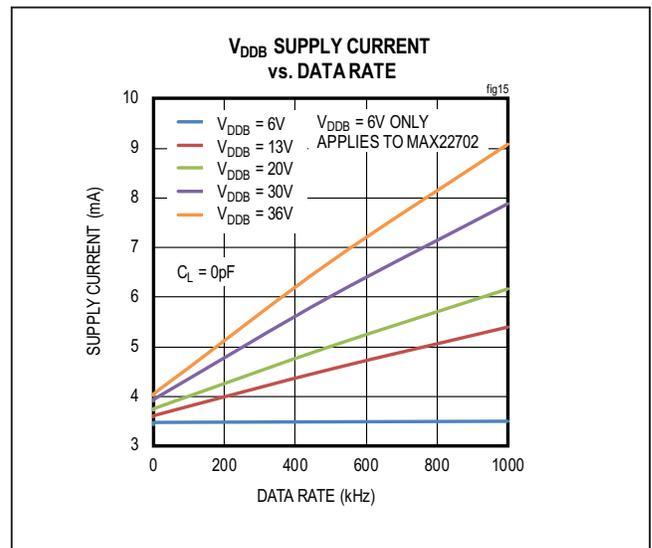
Figure 15.  $V_{DDB}$  Supply Current vs. Data Rate (typ)
