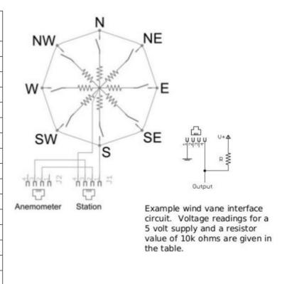
The wind vane is the most complicated of the three sensors. It has eight switches, each connected to a different resistor. The vane's magnet may close two switches at once, allowing up to 16 different positions to be indicated . An external resistor can be used to form a voltage divider , producing a voltage output that can be measured with an analog to digital converter, as shown below.
