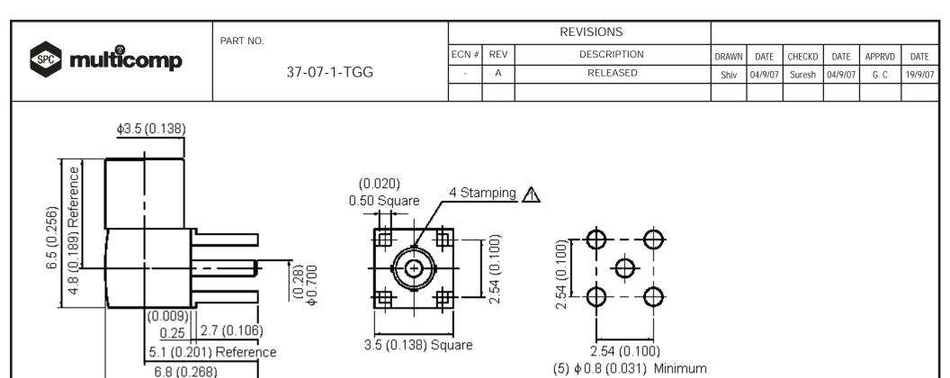
Mounting Hole Dimensions : Millimetres (Inches)
