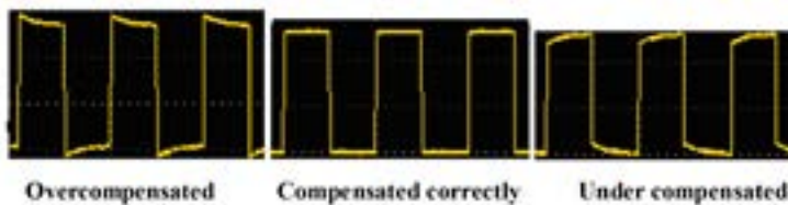
Figure 3-6 Displayed Waveforms of the Probe Compensation
