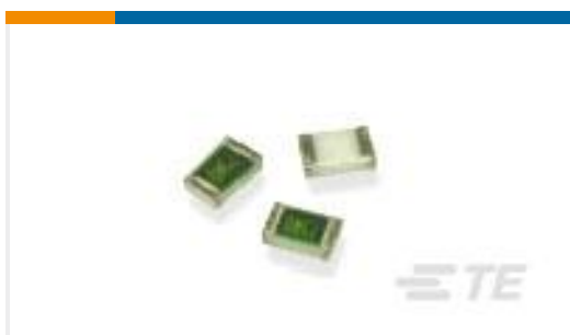
TE Part #5-2176091-2 RP 2A 0.25W 196R 0.1% 25PPM 1K RL
