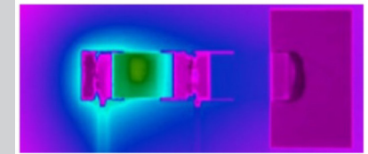
Ceramic Chip Resistor With Thermal Jumper (95.5 °C)
