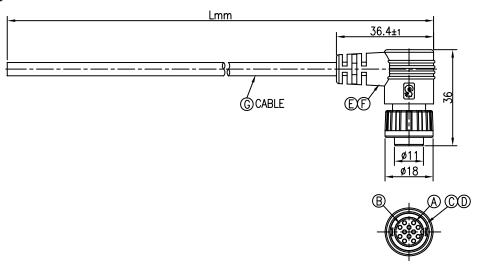
Dimensions: Millimetres CONN. WATERPROOF RATE: IP67
