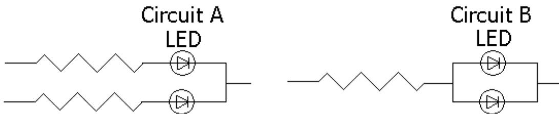
(a) Circuit A: it is recommended circuit.
