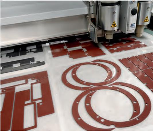
CAD data as a dxf file can be realised directly in ready and zero-toleranced exact cut templates without tooling costs. The outstanding production speed and a cutting technology perfected to the last detail provide an optimal result.
