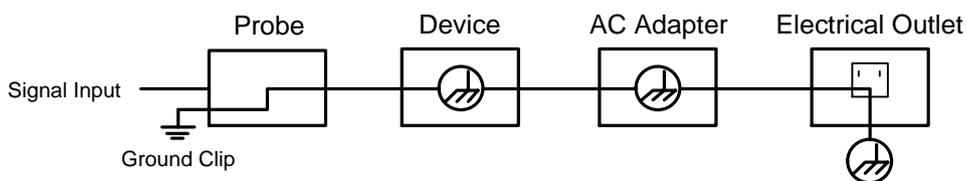
When the device communicating with PC via USB communication interface (with PC powered by AC power source), the illustration of the ground wire connection -
