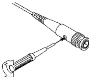
Figure 7-3. Probe Screw Adjusting
