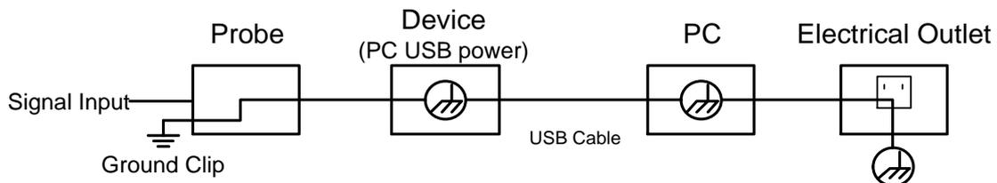
It is NOT allowed to measure AC power when the device been powered by AC power source through the adapter, or when the device powered by PC USB connection cable (via USB communication interface of PC, with PC powered by AC power source).
