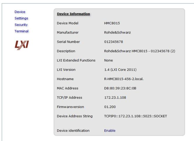
Fig. 10.12: Display of the device information
