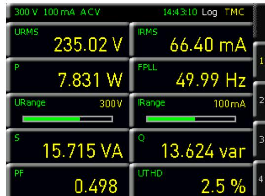
Fig. 5.5: Readout display with 10 active cells.
