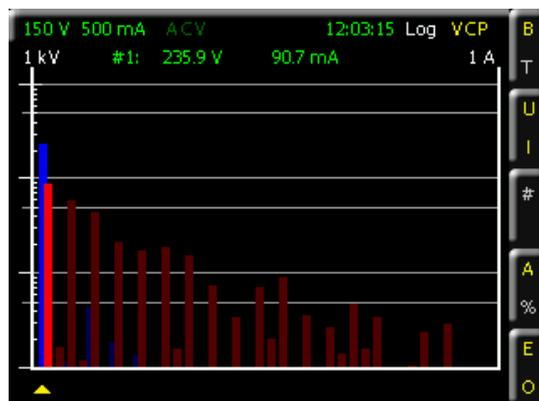
Fig. 6.4: Logarithmic readout display in Harmonics mode.
