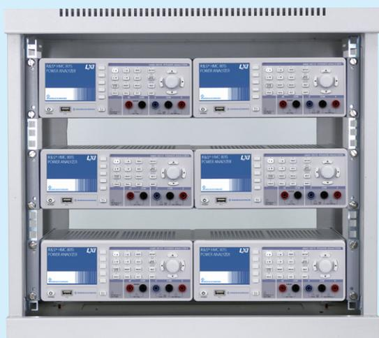
The instrument may be operated at an altitude of up to 2000 m. The specifications and tolerances apply after a warm-up time of at least 60 minutes, at an ambient temperature of 23 °C (± 2 °C). All values stated without tolerances are typical values for an average unit.
