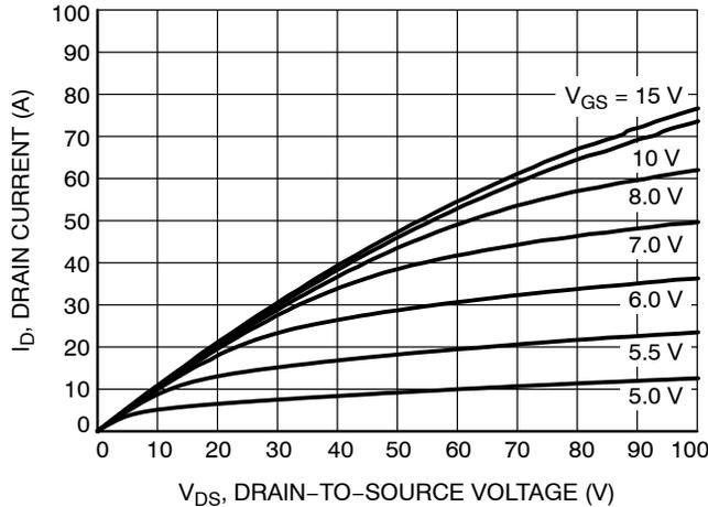
Figure 9. Saturation ( $150^{\circ}\text{C}$ )
