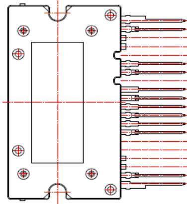
Figure 1. Pin Configuration
