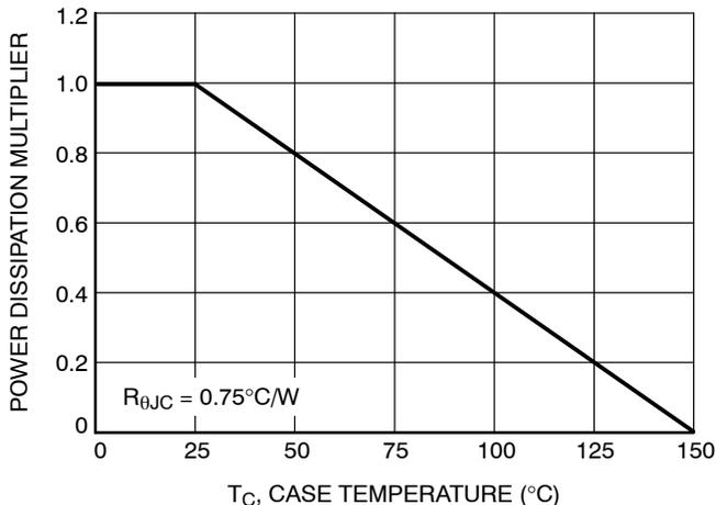
Figure 4. Normalized Power Dissipation vs. Case Temperature
