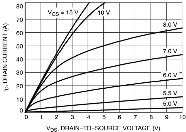
Figure 8. Saturation ( $25^{\circ}\text{C}$ )
