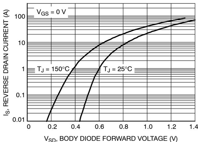
Figure 7. Forward Diode
