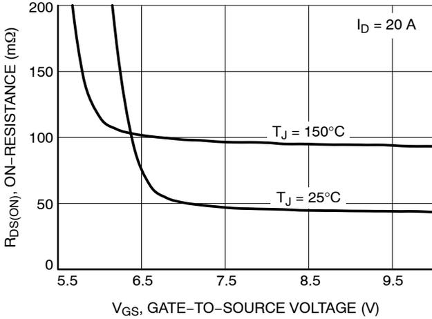
**Figure 10. On-Resistance vs. Gate-to-Source Voltage**
