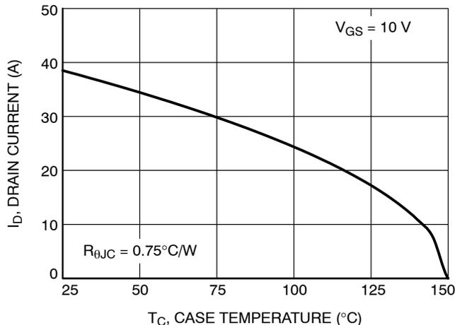
Figure 5. Maximum Continuous  $I_D$  vs. Case Temperature
