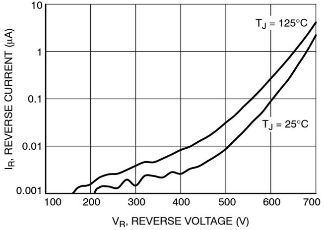
**Figure 22. Typical Reverse Current vs. Reverse Voltage**
