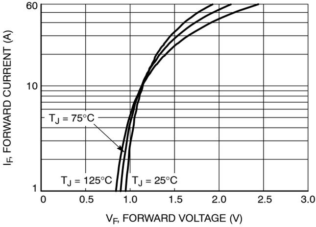
**Figure 21. Typical Forward Voltage Drop vs. Forward Current**
