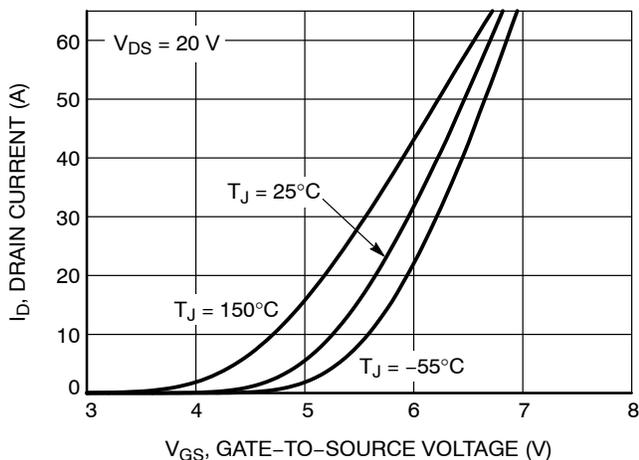
Figure 6. Transfer Characteristics
