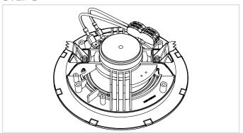
Bend the spring loaded mounting arms inwards by pushing them by fingers, making them fit through the provided ceiling cut-out.
