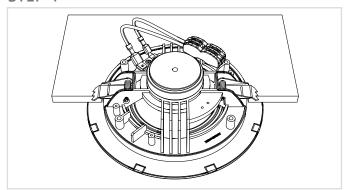
Insert the speaker through the provided ceiling cutout, make sure the spring loaded mounting arms are behind the clamping surface and release them. The ceiling is clamped between the mounting arms and the speaker baffle.
