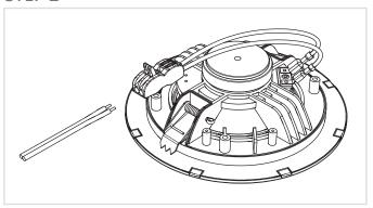
Connect the wires coming from the amplifier to the SnapConnect™ on the loudspeaker.
