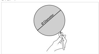
Cut a hole at the desired mounting location in the ceiling. Make sure the dimension is matching the cut-out measurement for the installing loudspeaker
