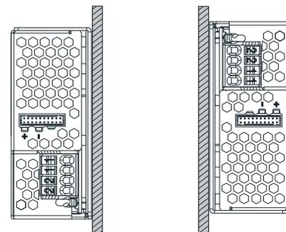
If the PSU is horizontal, upside down or side mounted, no derating is required.
