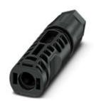
Photovoltaic connector, Range of articles: PV-CF-C, Photovoltaic connector, housing material: PPE, color: black, number of positions: 1, min. conductor cross section: 2.5 mm², max. conductor cross section: 6 mm², nom. voltage: 1500 V, rated current: 27 A, Connection method: Crimp, Type of contact: Pin, min. cable diameter: 5.00 mm, max. cable diameter: 8.00 mm
