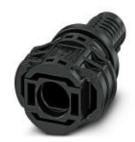
Photovoltaic connector, Range of articles: SUNCLIX, Photovoltaic connector, housing material: PPE, color: black, number of positions: 1, min. conductor cross section: 2.5 mm², max. conductor cross section: 6 mm², nom. voltage: 1500 V, rated current: 26 A, Connection method: Crimp, Type of contact: Plug
