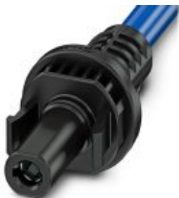
Photovoltaic connector, Range of articles: SUNCLIX, Photovoltaic connector, housing material: PPE, color: black, Connection method: Crimp, Type of contact: Socket
