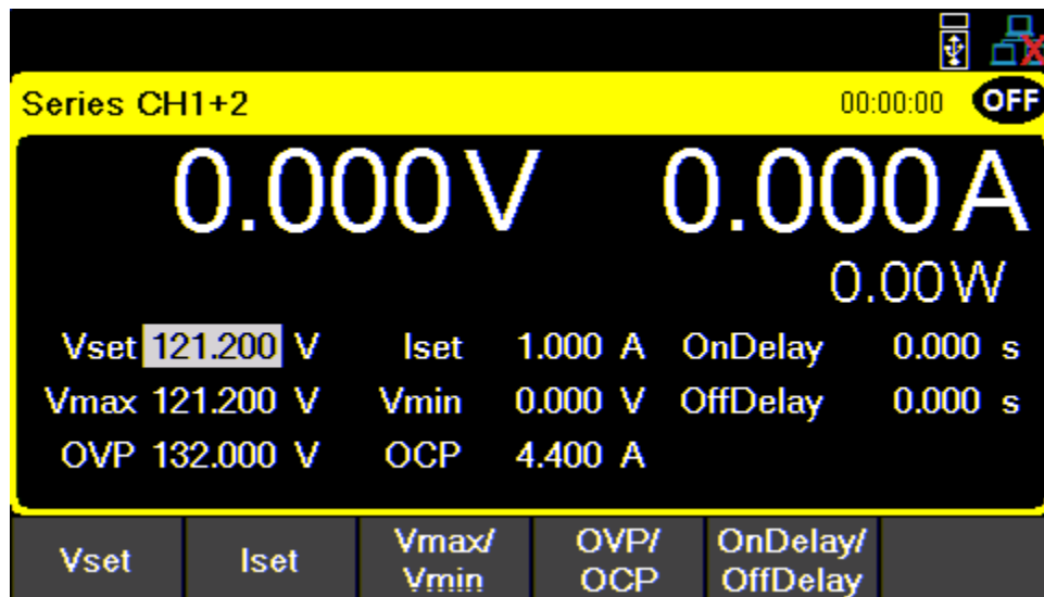
Figure 4.8 Series CH1+2 Single Channel Display
