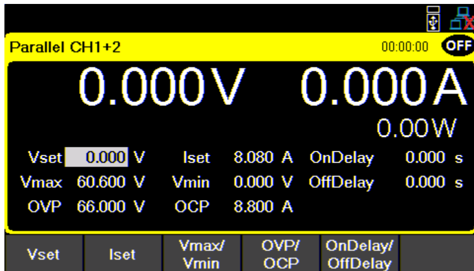
Figure 4.14 Parallel CH 1+2 Single Channel Display
