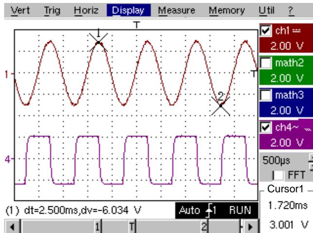
**Composition** The oscilloscope display is divided into 4 functional zones.
