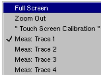
By double-tapping with the stylus in the display area, the menu concerning the display can be opened directly.
