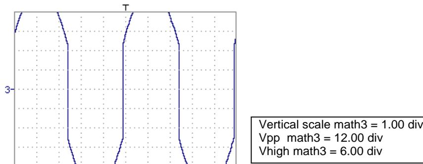
There is a high and low overshoot, so division by 2 is necessary to optimize display of the result.
