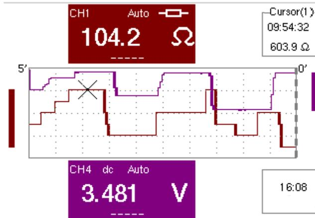
☞ The screen display is identical if CH1 is configured for amplitude measurement, as an ohmmeter or for temperature measurement (PT100).
