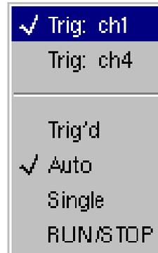
RUN/STOP starts and stops acquisition from this menu. The acquisition status is indicated in the status area on the screen.
