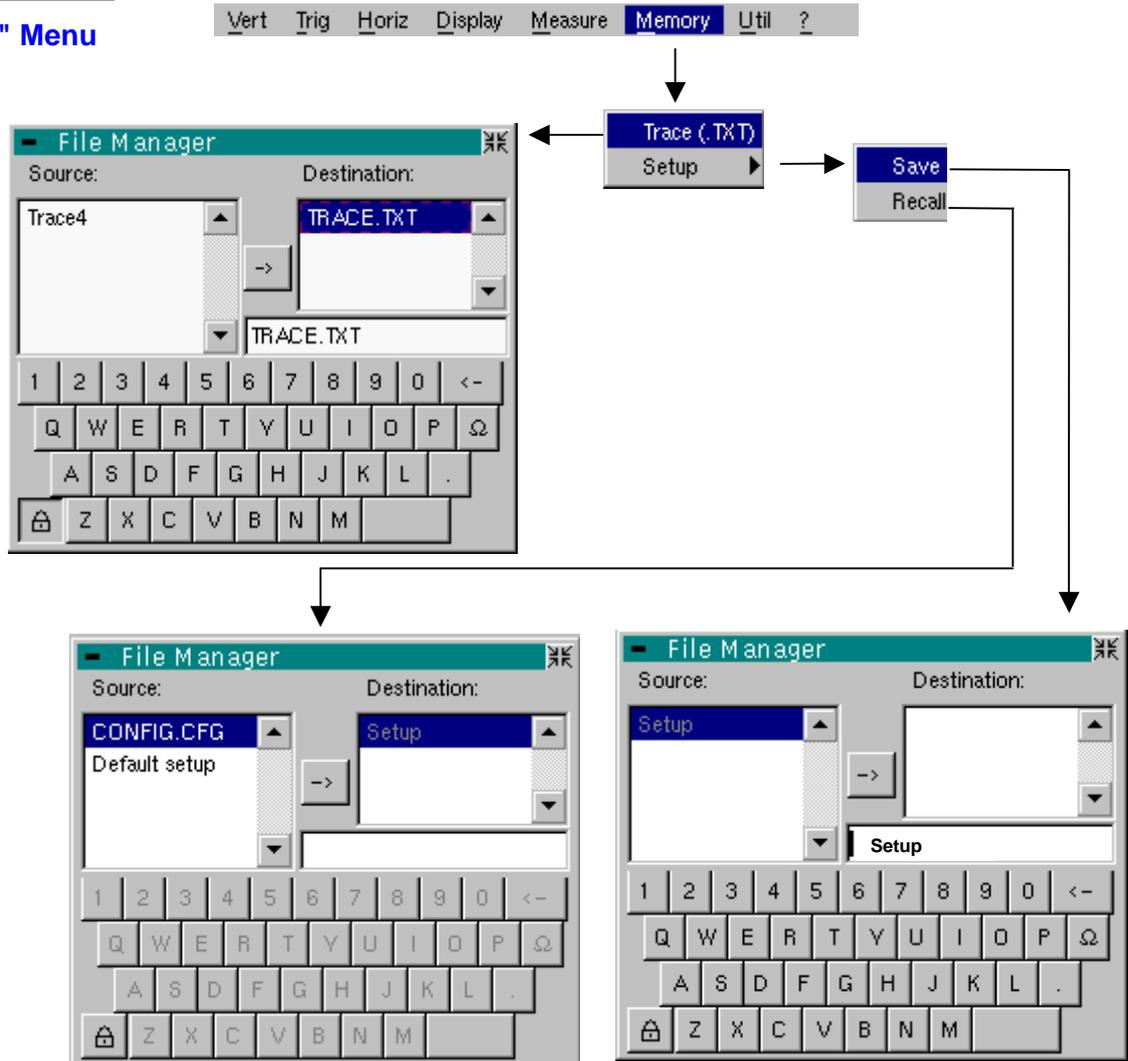
**Trace (.TXT)** In "Multimeter" mode, it is only possible to save a trace in non-volatile memory in .TXT format. Files saved with the suffix .TXT can be exported onto a PC (see §. Util Menu → Files) for processing with other software (spreadsheet, etc.).
