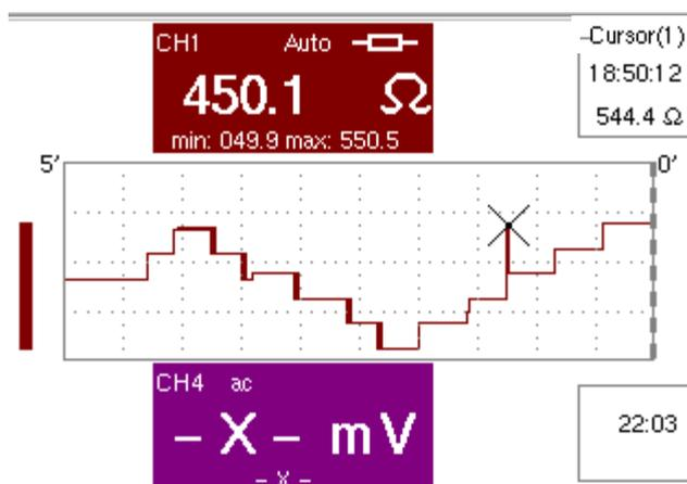
The graphic window records the changes in the measurements during the analysis period (5 minutes).
