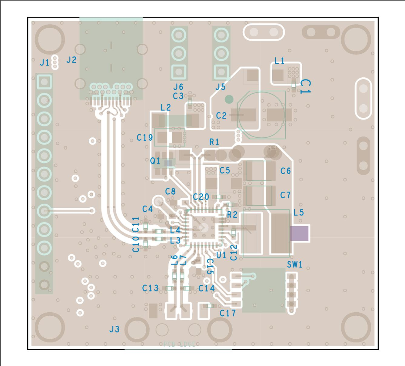
MAX20461 EV Kit PCB Layout—Top View
