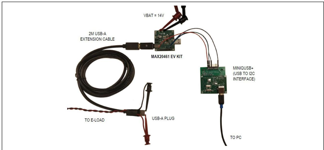
Figure 6. Cable Compensation Setup
