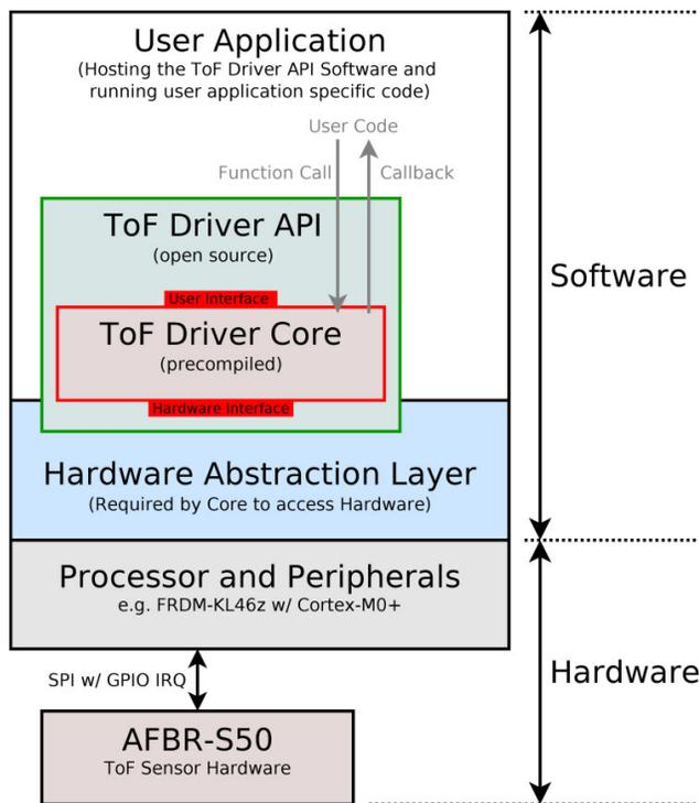
Figure 13 shows the software architecture overview for the basic implementation of the ToF Driver Core into user hardware and software. The precompiled core is embedded into open source API layers, providing an interface to the user application. A hardware interface declares the required hardware access for the ToF driver core to the underlying hardware and peripherals. The latter is required to connect the core to the AFBR-S50 ToF sensor hardware through the SPI and GPIO interfaces.
