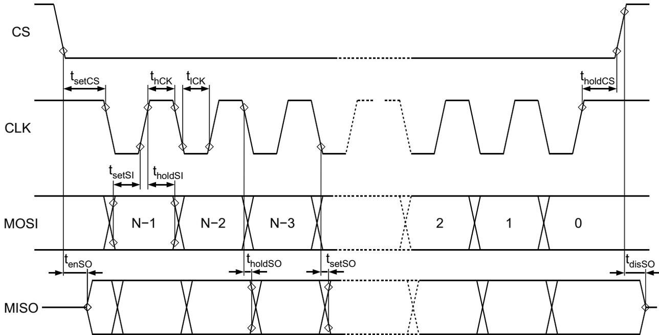
Table 6: SPI Slave Interface Timing Parameters
