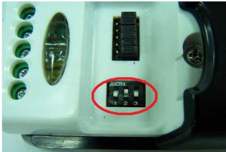
**Figure 2 - 3-Pin DIP Switch for Operating Mode Selection**
