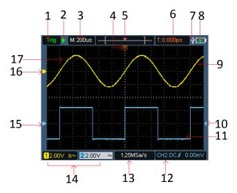
Figure 5: Oscilloscope Interface
