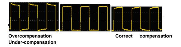
Figure 0-2: Display Waveform of Probe Compensation
