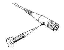
Figure 0-3: Probe Adjustment
