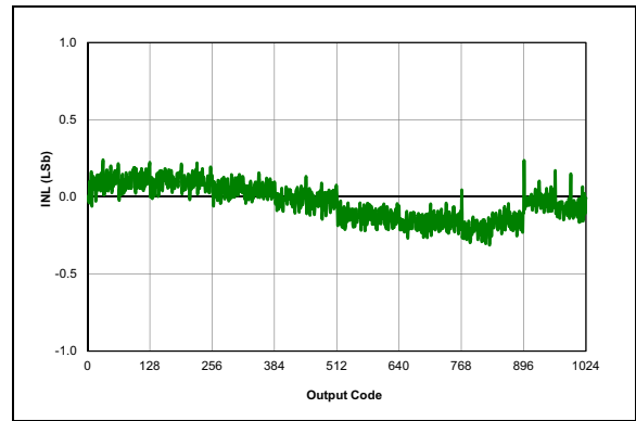
FIGURE 38-35: ADC, INL, V_{DD} = 3.0V , T_{AD} = 1\ \mu\text{S} , 25^\circ\text{C} .
