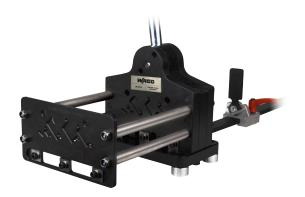
WAGO now offers options for panel shops and machine builders to cut and punch their own custom size DIN rail. There are three variations of the DIN rail cutter: a standard option with manual operation, a universal option (capable of 5 different sizes/types of rail and vertical and horizontal punches) with manual operation, and an automated version of the universal cutter with air over hydraulic cylinder. Additionally, a wire duct/channel cutting option is available.
