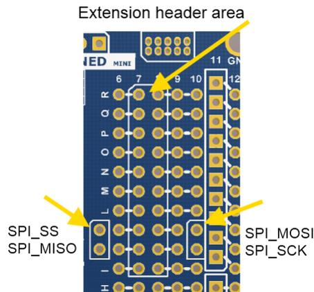
The SPI bus signals are available close to the header at row J and K, enabling easy connection to header pin 15 to 18.
