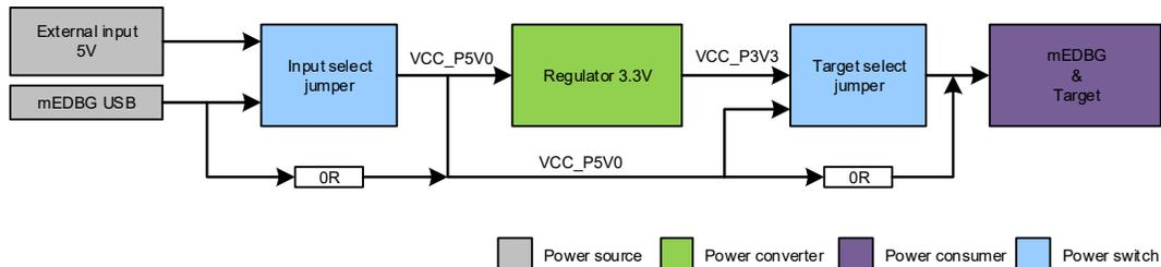
The input voltage select jumper (J300, 3-pin header footprint) can be soldered in to select between power from the USB port or the VIN pin on the Arduino power header footprint. By default, the selector is bypassed with a 0Ω resistor (R300) to connect the USB voltage to the on-board 3.3V/150 mA regulator and target voltage select header.
