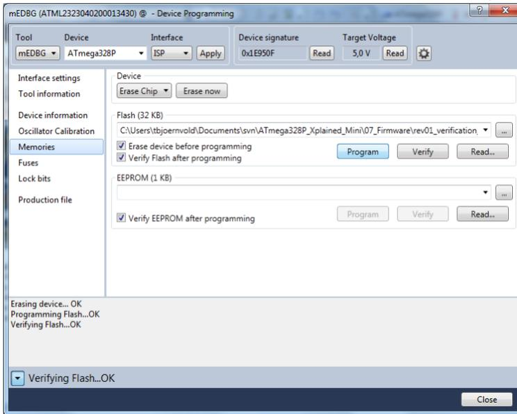
4. **NOTE:** If a previous debug session was not closed by selecting “Disable debugWIRE and Close” in the Debug menu, the DWEN fuse will be enabled, and the target will still be in debug mode, i.e., it will not be possible to program the target using the ISP interface.
