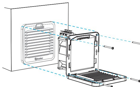
The installation with the only clips is optimized for 1.5 mm thick sheets; it is also possible with thicknesses from 1 to 2.5 mm. Fixing with screws (supplied) is recommended. Tightening torque 0.3 Nm.
